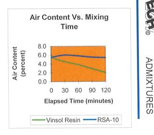
\*Test based on lab results with ambient temperatures between 62 F (17 C) and 70 F (21 C). Plastic concrete was adjusted to maintain slump at fifteen minute intervals. At each interval, air was checked using ASTM C 231. Slump was measured using ASTM C 143. Air contents are portrayed on the above graph.
