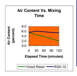
\*Test based on lab results with ambient temperatures between 62 F (17 C) and 70 F (21 C). Plastic concrete was adjusted to maintain slump at fifteen minute intervals. At each interval, air was checked using ASTM C 231. Slump was measured using ASTM C 143. Air contents are portrayed on the above graph.
