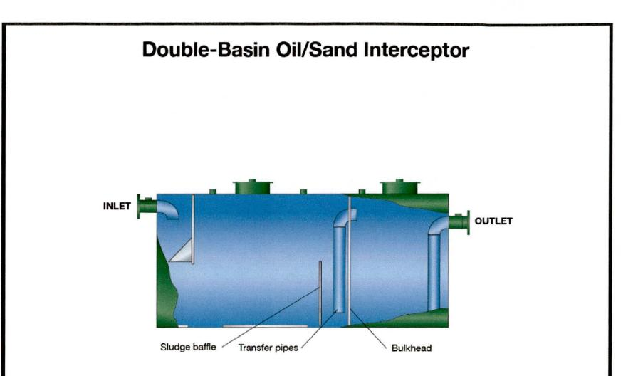
Double Basin Interceptors have two collection chambers and a sludge baffle. They are commonly used in car wash and commercial or municipal vehicle washing applications for oil and sand removal prior to discharge to a recycle wash system. An optional overflow bypass directs excess flow to an auxiliary retention area.
