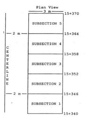
Multiply the width of the test section by the random numbers for the width. 1. 3.00 x .222 = 0.7 2. 3.00 x .036 = 0.1 3. 3.00 x .791 = 2.4 4. 3.00 x .966 = 2.9 5. 3.00 x .747 = 2.2
