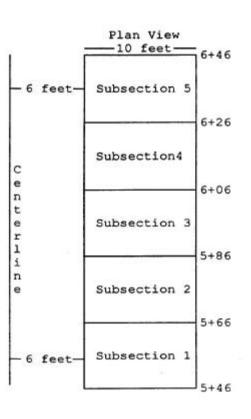
Multiply the width of each subsection by the random numbers for the width.
