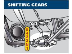
squeeze the clutch lever, 2) lift the shift lever firmly as far as it will go and release, 3) smoothly ease out the clutch lever and adjust the throttle.
