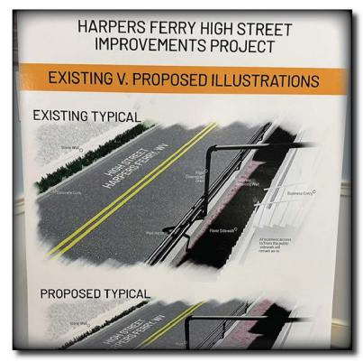
The scope of the project includes 291 linear feet of work along the north side of High Street between Hog Alley and Public Way. It would shift roadway alignment between the two streets two feet to the south, and widen the existing sidewalk equivalently. Included with that would be a new 12-inch-thick retaining wall, and metal railing.
