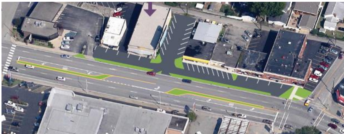
Potential consolidation and elimination of curb cuts
