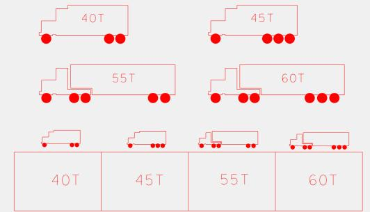
The maximum allowable Gross Vehicle Weight (GVW) in tons for each of four vehicle types is shown above. Four boxes are shown adjacent to each bridge, corresponding to the above four vehicle types. A number in any box indicates a posted load less than the maximum allowable. A blank box indicates the bridge limit will be the maximum allowable GVW.
