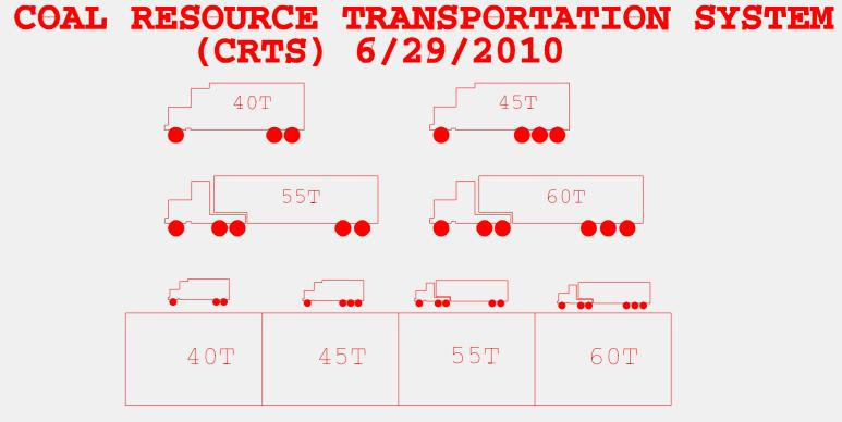
The maximum allowable Gross Vehicle Weight (GVW) in tons for each of four vehicle types is shown above Four boxes are shown adjacent to each bridge, corresponding to the above four vehicle types. A number in any box indicates a posted load less than the maximum allowable. A blank box indicates the bridge limit will be the maximum allowable GVW.
