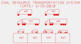
The maximum allowable Gross Vehicle Weight (GVW) in tons for each of four vehicle types is shown above. Four boxes are shown adjacent to each bridge, corresponding to the above four vehicle types. A number in any box indicates a posted load less than the maximum allowable. A blank box indicates the bridge limit will be the maximum allowable GVW.
