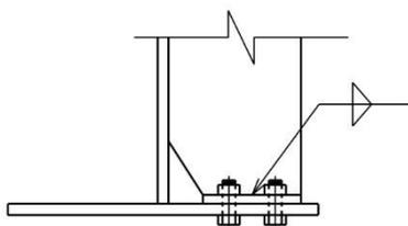
ALTERNATE DETAIL AT TENSION FLANGE WHERE STRESS RANGE EXCEEDS CATEGORY C
