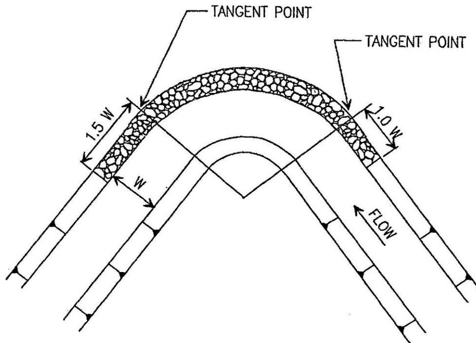
As shown in Figure 7-6, the minimum upstream distance should be equal to the channel width and the minimum downstream distance should be at least 1.5 times the channel width from the corresponding tangent points. This guidance is based on studies of a symmetrical channel bend under ideal laboratory conditions. Real-world conditions are rarely as simplistic and the distances should be increased to reflect site conditions.
