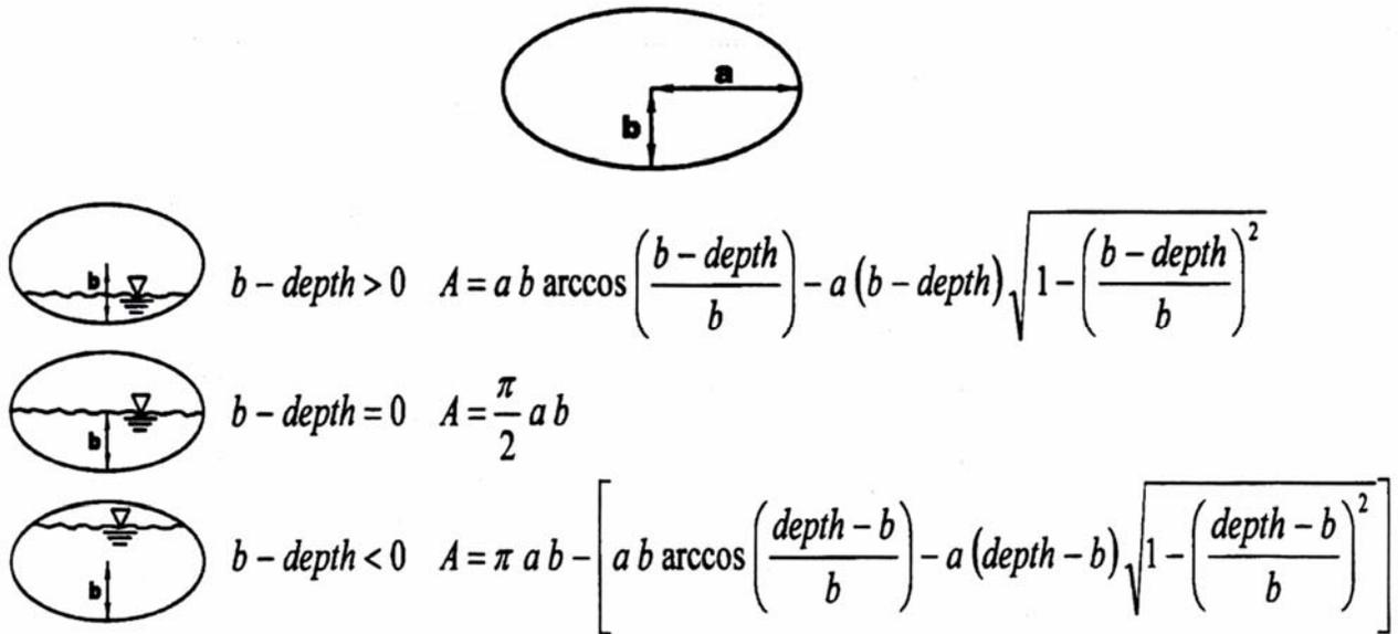
This chart provides equations for calculating the flow area for any flow depth within an elliptical pipe. It can be useful for calculating the critical depth of flow using the critical depth equation (see Section 8.4.5.1).
