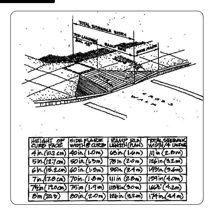
Curb ramp run as a function of curb height
