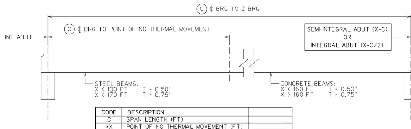
\*THE POINT OF NO THERMAL MOVEMENT SHALL BE COMPUTED USING BEST ENGINEERING PRACTICE FOR MULTI SPAN BRIDGES.
