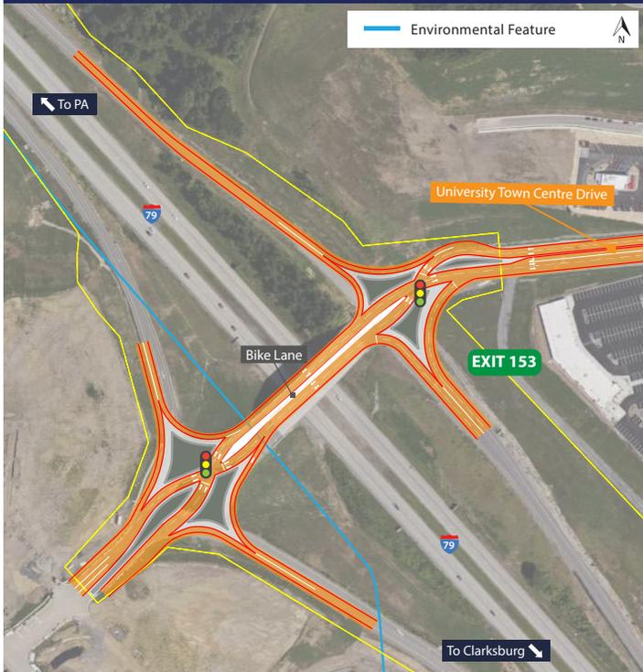
**Alternative 3 converts the existing interchange to a diverging diamond interchange (DDI). This is the recommended alternative. More information is provided on the DDI board and in the video.**
