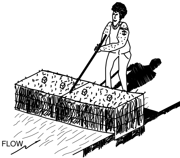
3. WEDGE LOOSE STRAW BETWEEN BALES
