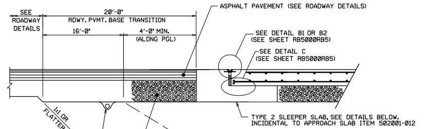
TYPE 2 SLEEPER SLAB WITH ASPHALT ROADWAY APPROACHES
