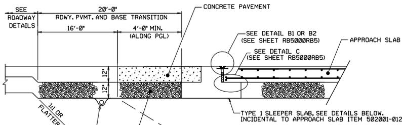
TYPE 1 SLEEPER SLAB DETAIL WITH CONCRETE ROADWAY APPROACHES
