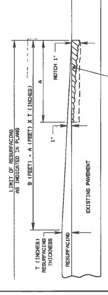
WHEEL RUTS BEYOND THE HEEL-IN NOTCH AME TO BE FILLED AND TRANSITIONED TO MEET FIELD CONDITIONS.
