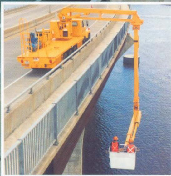
Particular attention has been given to traffic control problems. The ASPEN AERIALS UB units afford stability without outriggers and the rotating counterweight stays within the 96" (2436 mm) width of the truck body thus keeping any portion of the unit from occupying more than one lane of traffic!
