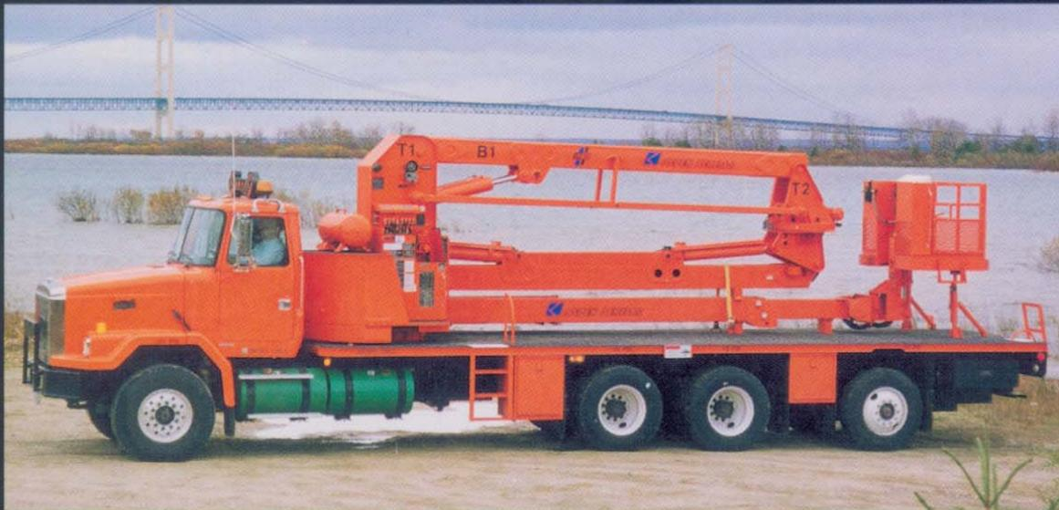
The Model UB50 in the traveling position.
