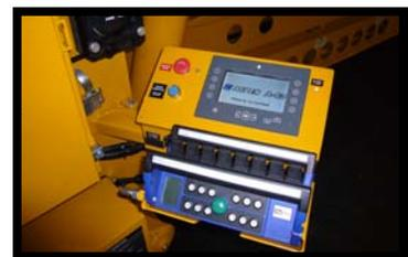
As the most advanced microprocessor control system available, the “Plus 1” Graphical Terminal Interface includes a color display depicting unit operation and individual function performance while monitoring the unit’s parameters, hydraulics and enabling simple troubleshooting. Wireless controls are included at both operator stations.
