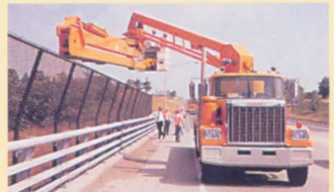
**VERTICAL BARRIER CLEARANCE** - designed to deploy over fences in excess of 10 feet.
