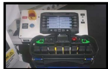
As the most advanced microprocessor control system available, the "Plus 1" Graphical Terminal Interface includes a color display depicting unit operation and individual function performance while monitoring the unit's parameters, hydraulics and enabling simple troubleshooting. Wired/Wireless type controls are included at both operator stations.
