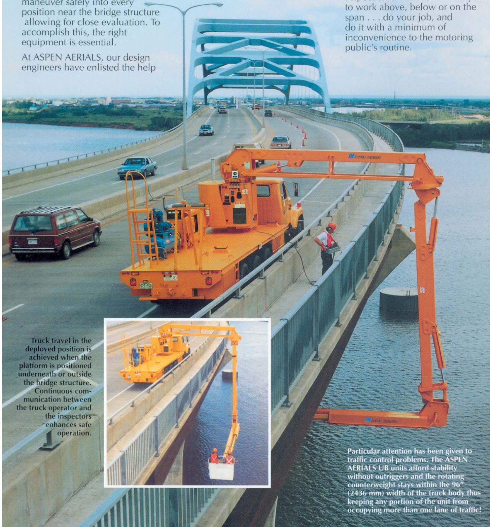
Truck travel in the deployed position is achieved when the platform is positioned underneath or outside the bridge structure. Continuous communication between the truck operator and the inspectors enhances safe operation.
