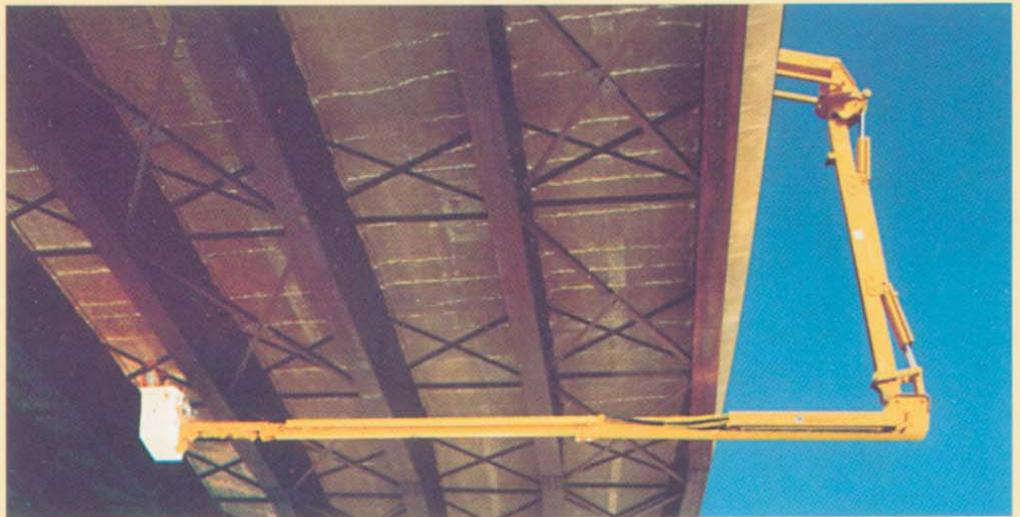
**EXTENDED REACH** - Up to 60' (18.3 m) of underbridge working reach available without requiring that the truck chassis be repositioned.
