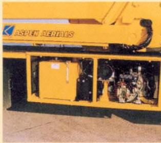
**TWO POWER SOURCES** are provided. The primary source of power is a power-take-off from the truck transmission. A liquid-cooled diesel engine capable of powering the Bridge Inspection Unit is provided as backup.
