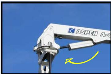
Turntable no. 2 comes equipped with an automatic leveling system, providing smooth platform movement. In addition, the operator can make manual adjustments of +/- 5 degrees to compensate for the slope of the bridge. With the elimination of the leveling arms, the Aspen A-62 has more vertical clearance to get over high fences.
