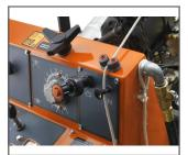
**CLAM CLEAT POINTER ROPE HOLDER** Reduces pointer rope damage and holds front pointer at a set height.
