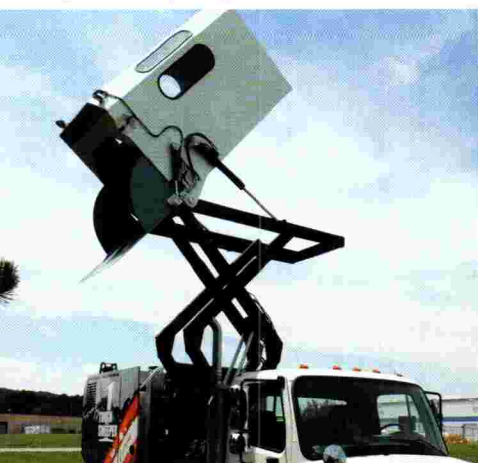
49" Diameter Side Broom(s) with Gutter Broom Extension Override.
