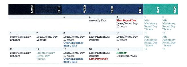
To determine the low bidder, the WVDOH will calculate the Large Crane Lease/Rental rate, both weekly and monthly for this example. WVDOH also calculates in the Idle Machine Rental rate and Overtime rate, roundtrip Mileage, Assembly fee and Disassembly fee for each Vendor.
