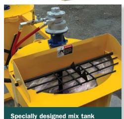
provides high shearing action for thorough and complete particle
