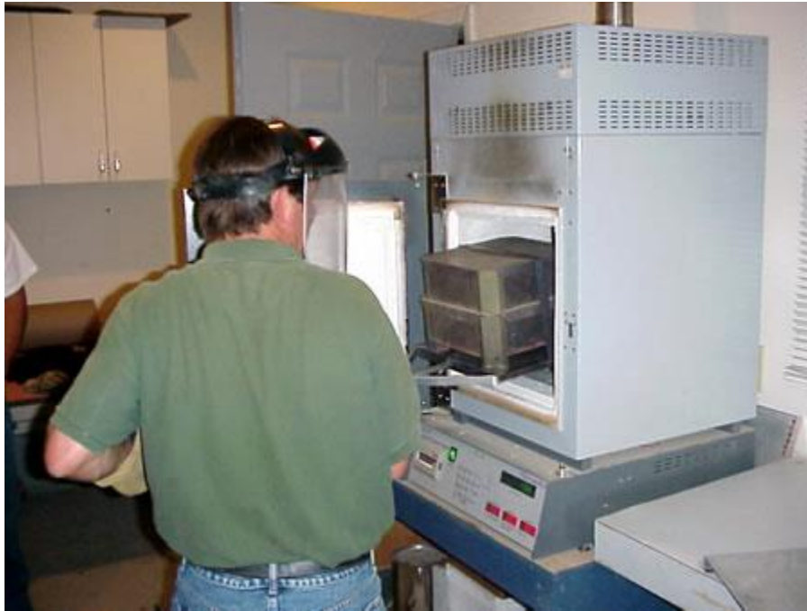
Figure 50 - Determining Asphalt Content using NCAT Ignition Oven
