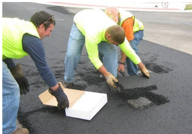
Figure 41 - Roadway Plate Sampling
