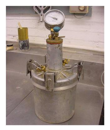
This test method describes the procedure for determining the air content of freshly mixed concrete by observing the changes in volume caused by changes in pressure. The standard procedure for conducting this test is AASHTO T 152. This method is intended for use with concrete and mortar made with relatively dense natural aggregates. It is not to be used with concrete made with lightweight aggregates, air-cooled blast-furnace slag, or aggregates of high porosity.
