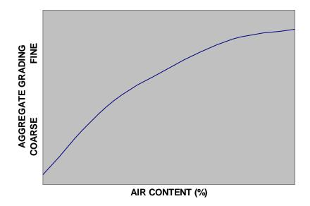
Since the air is entrained in the mortar fraction of the concrete, the coarser aggregate particles have little effect on the air content.
