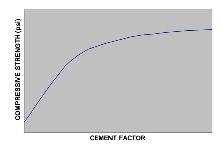
The cement factor (how many pounds of cement per unit volume of concrete) has the greatest affect on the strength of Portland cement concrete.
