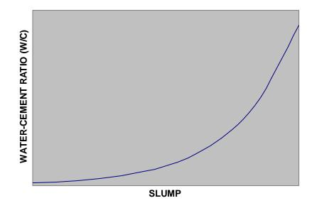
As you can see in the chart, as the water cement ratio increased the slump also increases. Once the slump gets to a point where it is not measurable, an increase in the W/C Ratio has no measurable effect. A general rule of thumb is: For each three percent increase in water, you can expect a one-inch increase in slump. The reverse also holds true; if the water decreases by three percent, the slump will decrease approximately one-inch.
