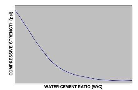
As the water cement ratio increases, the strength decreases. This is the first in a chain of properties that affect each other, and ultimately affect the strength.
