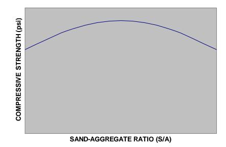
The sand-aggregate ratio can be either too high or too low for optimum strength.
