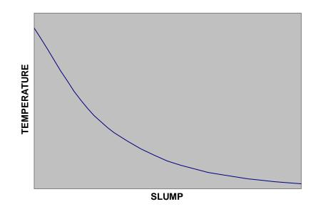
As the temperature of the concrete increases, the slump will decrease. This might also be stated: as the temperature of the concrete increases, the amount of water needed to maintain a constant slump would increase.
