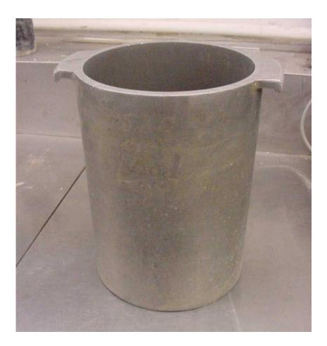
One of the characteristics of Portland cement concrete that can be used as a very useful tool is the unit weight (weight per cubic foot). Unit weight (or weight per unit volume) is generally expressed as pounds per cubic foot and is written as lb/ft<sup>3</sup>.
