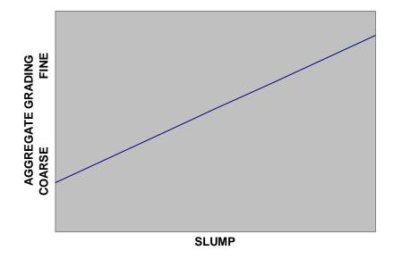
Concrete with a given amount of water will become more plastic (higher slump) as the grading becomes finer. Of course there is a limit to the effect extra fines will have on the slump.
