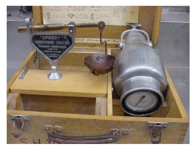
The speedy moisture test is a fast way to get the moisture content of the fine aggregate to be used when batching concrete. It is a useful test at the batch plant, but also, it can be useful in the field such as when mobile mixers are used to batch concrete. It can be very helpful to know how to perform this test, but it is no longer one of the tests on which a PCC Inspector candidate will be tested. The procedure for performing a speedy moisture test is as follows:
