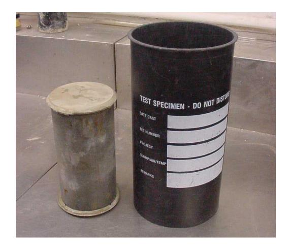
The compressive strength of concrete is expressed as the load (in pounds) per unit area (square inches) that would be necessary to crush the concrete. The common procedure used to measure the compressive strength of concrete is to place a sample of the concrete (called a test cylinder) in a testing machine and find the force required to crush it.
