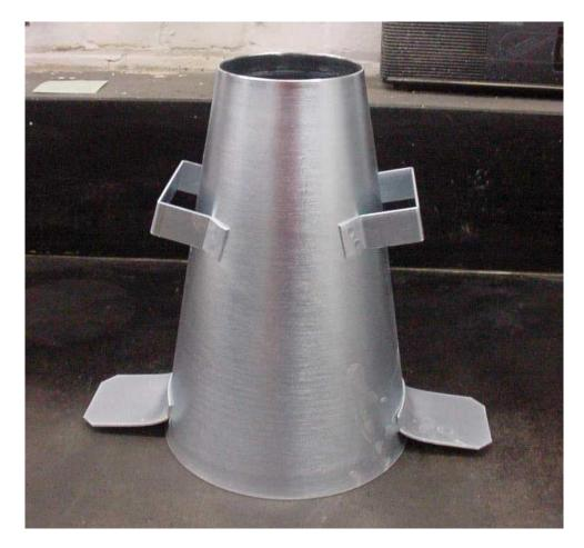
The consistency of Portland cement concrete is a measure of the freshly mixed concrete's ability to flow. This property is important because concrete must have the proper consistency and workability for different applications. For example, a higher slump concrete (more flowable) would be desirable when reinforcing steel is spaced close together or when concrete is being placed by pumping.
