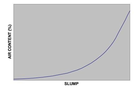
As the air content of the concrete increases there will be a corresponding increase in slump.
