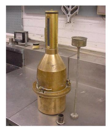
This method of test covers the procedure for determining the air content of freshly mixed concrete containing any type of aggregate, whether it is dense, cellular, or lightweight.
