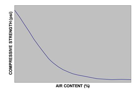
As the air content of concrete increases, the strength of the concrete decreases. Some entrained air is needed in concrete for the purpose of freeze-thaw resistance and possibly other factors. A balance must be achieved between the desired strength and the desired entrained air content.
