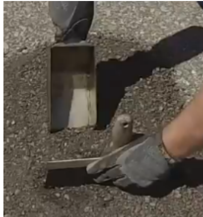
Figure 40 - Roadway Scoop Sampling
