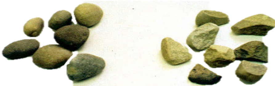
Figure 16 - Difference between river gravel before and after crushing
