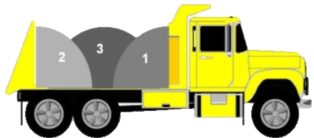
Figure 30 – Correct Truck Loading Scenarios
