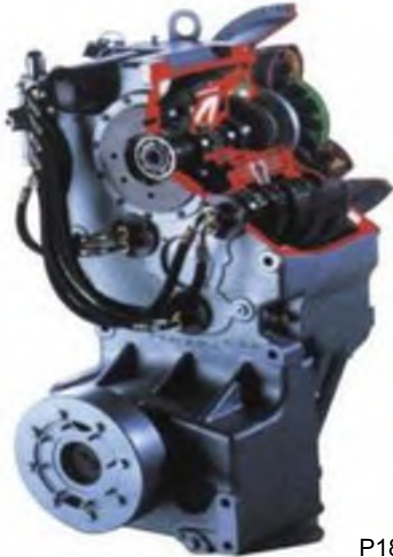
Figure 3-7 External view of torque converter - gear box assembly
