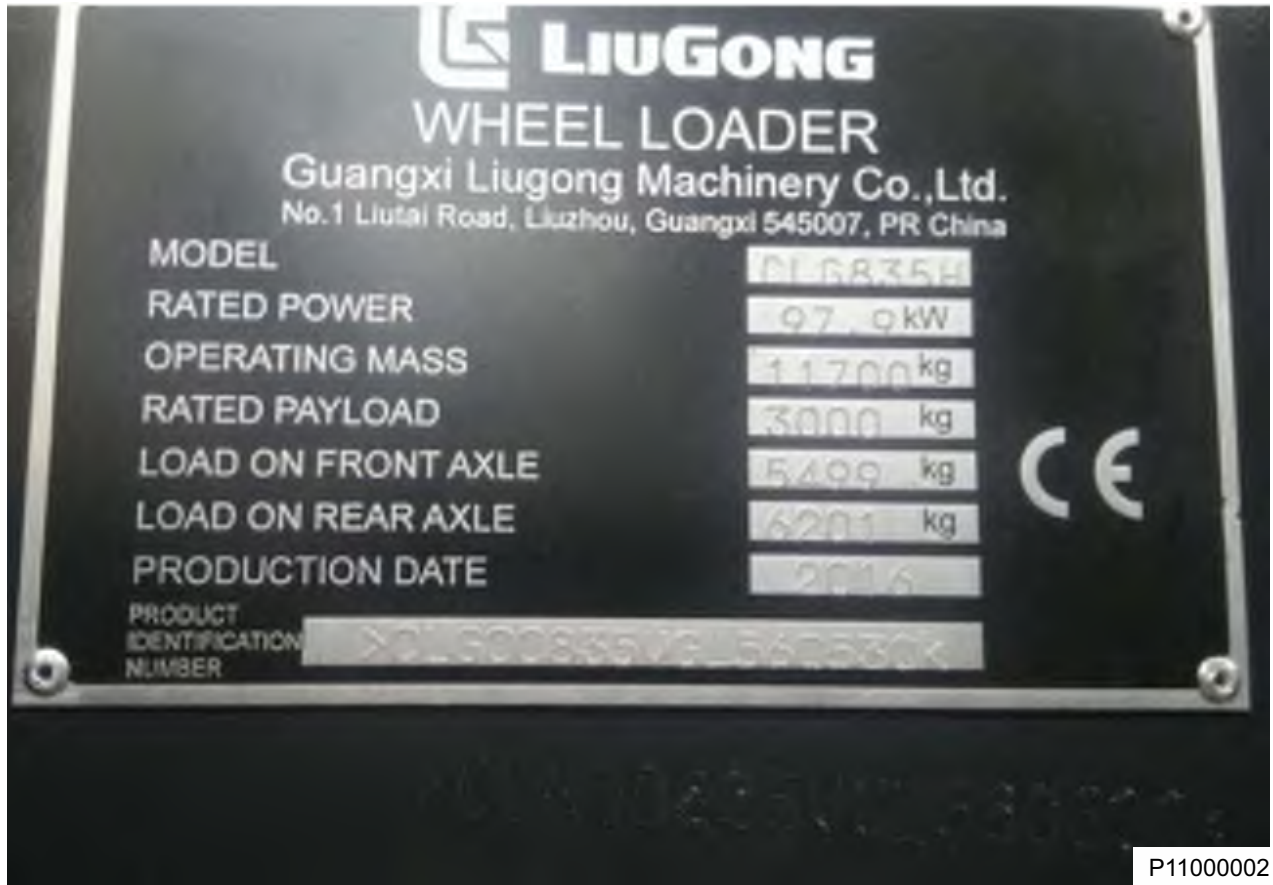
Figure 2 Pin Plate (17-character with CE mark)
