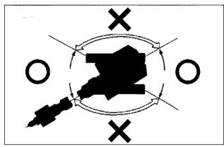
Operate the excavator carefully to avoid hitting the boom with the hydraulic breaker.
