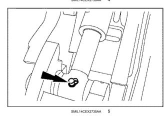
**NOTICE:** the coupler linkage shall be lubricated every **10 h** if the machine is operated in water or mud.
