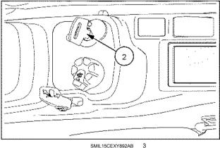
7. Remove the starter key, get off the cab and lock the cab door. Check that the hood and the side doors are properly locked, and that the lower panels are properly fixed.
