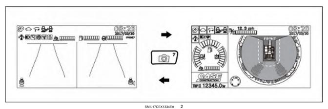
**NOTICE:** During machine operation, make sure to select either one operating mode of the display in order to ensure proper visibility around the machine. If the display is switched to the user information mode during machine operation, the warning message SELECT CAMERA SCREEN DURING OPERATION will appear on the top of the display.
