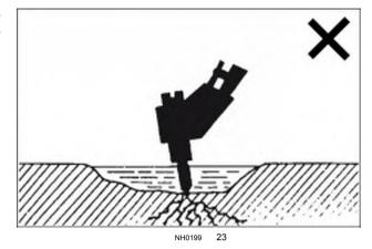
Do not use the hydraulic breaker to move objects. The excavator might overturn and/or the hydraulic breaker may be damaged.
