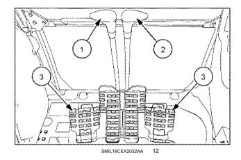
The travel control levers and pedals are used to move the machine.
