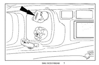
2. Set the gate lock lever in unlock position.
