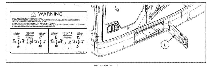
4. Pull the knob (1) and move the lever (2) to set the lever to the desired operation pattern C or D.
