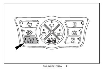
The tab for operational settings of the auxiliary high-flow hydraulic circuit features two pages. These two pages allows to set and store specific flow rate/pressure combinations according to the type and to the specifications of the attachment used.
