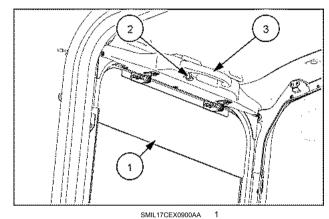
3. Pull the windshield to the rear until it engages perfectly behind the cab.
