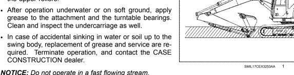
**NOTICE:** Do not operate in a fast flowing stream.
