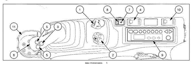
(1) Starter switch (4 positions): ON (contact), START (engine ignition), OFF (engine shut-down) and ACC (accessory current supply).
