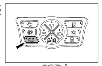
8. Select the breaker page and set the proper flow rate/ pressure combination.
