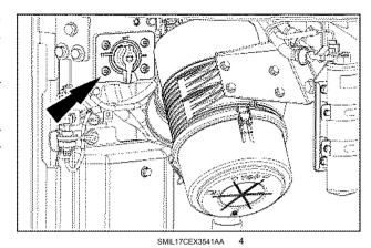
The battery disconnect switch shall be in ON position for normal operation.
