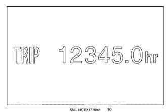
The hour meter is displayed by default. To display the trip meter, press the hour meter button: the trip meter will be thus displayed for approximately **1 min**, after which the hour meter will be displayed again.
