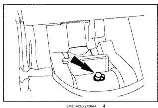
• Cylinder top pin: one lubrication point.
