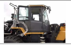
Pull the latch unlocking handle to unlock the window, and then pull the inner handrail backward to close the right window.
