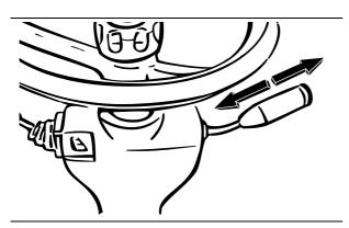
The washer will work by pressing the washer control switch inwards. The water from reservoir will be sprayed to windshield window glass.
