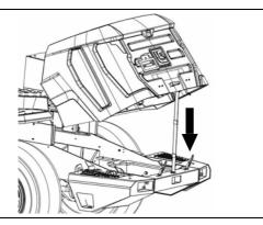
2. Pull the fasteners on the left and right sides of the rear door upward to lock the engine hood.
