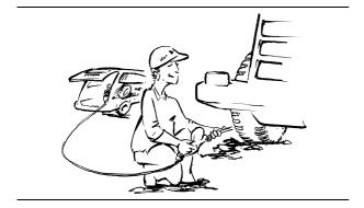
Explosions of tires have resulted from gas heatinduced and combustion inside the tires. Explosions can be caused by heat that is generated by welding, by heating rim components, by external fire, or by excessive use of brakes.
