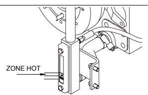
9. Start the engine and run at idle speed. Check the transmission oil level again and add the transmission oil until the oil level is above COLD ZONE. The transmission could produce a slightly abnormal noise due to transmission oil insufficiency. The abnormal noise will disappear after the transmission oil reaches the specified level.
