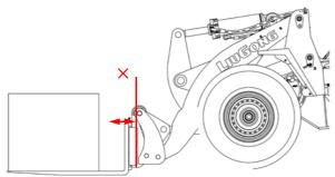
3. Slightly tilt the forks backward to get a better stable position for the material.
