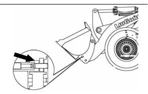
10. To ensure the coupler connecting pin is fully engaged into the work attachment, tilt the work attachment downwards onto the ground and apply slight force. Then raise the boom (about 1.5 m) and tilt the bucket forwards. Do not separate the bucket from the coupler frame.
