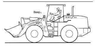
Only start the engine from the operators seat in the cab. The transmission should be in NEUTRAL position before engine starting. Never start the engine by short-circuiting the starter motor terminals. Starting the engine by shortcircuiting could result in damage of the electrical system, personal injury or death.
