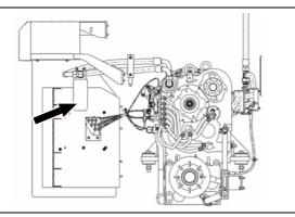
The secondary filter of ZF160 gearbox is located in the accumulator box. Secondary filter of ZF160 gearbox
