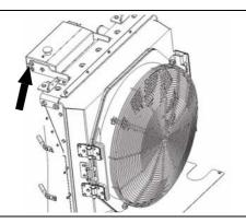
2. Check the coolant sight glass on the recovery tank. Add coolant if the coolant level is lower than the centerline of the sight glass.
