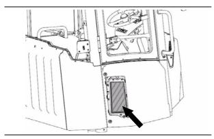
2. Clean the strainer with compressed air. If the strainer is too dirty or too oily, wash it with neutral detergent. Dry the strainer completely before reuse.
