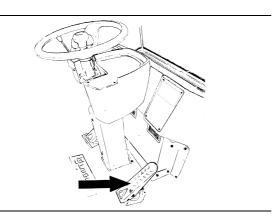
The accelerator pedal is located at the front right side of the driver's seat. The diesel engine oil supply and the engine speed will increase by depressing the pedal while the oil supply and the engine speed will reduce by releasing it.
