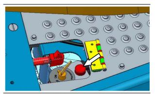
Cooling and purging of the DEF system will take place at the same time. Disconnecting the battery power too soon may prevent cooling of the DEF system and purging of the DEF lines after the engine is shut down, which can damage the DEF system. Only when the wait to disconnect lamp is extinguished should the battery disconnect switch be turned off.
