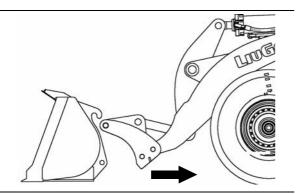
8. Push stop plate inwards to lock the auxiliary control lever. Then tighten nut of the lock.
