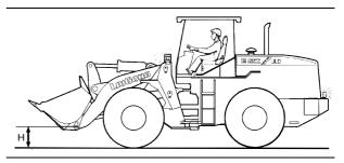
Depress the service brake pedal and press the parking brake button (or release the parking brake handle) to disengage the parking brake. Slowly release the service brake pedal and observe the machine for movement.
