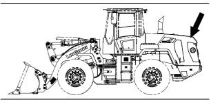
2. Remove the dust and debris on the radiator group by compressed air.
