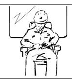
Ensure the hydraulic control levers are all in the NEUTRAL position and the shift control lever is in the NEUTRAL position before starting the engine.
