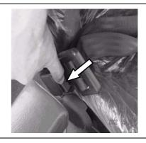
Before using the seat belt, check whether the buckle of the seat belt can lock and release normally.
