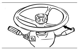
Articulate full-hydraulic power steering is provided on this machine, the steering wheel is in the cab and it is connected to the full-hydraulic metering pump through steering column. In normal operation, turn the steering wheel clockwise, the machine will turn right; turn the steering wheel counterclockwise, the machine will turn left.
