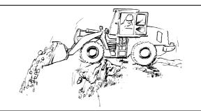
When driving the machine on a slope, make it straight up and down and neither make turn on the slope nor drive it transversely on the slope to prevent tipping. The distance between bucket and ground should be 200-300mm (7-12in).
