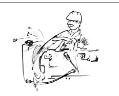
Wear relevant personal protective equipment (PPE) such as a hard hat, ear protection, safety glasses, safety shoes and gloves when operating or servicing the machine.
