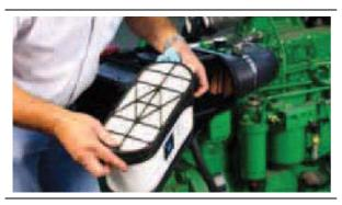
4. Take out the safety filter element. Use the handles on the safety filter element to pull it towards the filter housing center, and then take it out.
