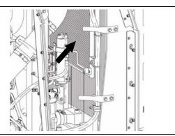
Clean the condenser regularly. Mainly need to clean the radiator fin of the condenser, too much dirt on the radiator fin will affect the condenser cooling and reduce its performance, and finally affect the cooling of the air conditioning system.
