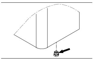
2. Remove return oil filter flange and O-ring, take out the element.
