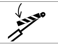
For those parts fitted with shields, if it is necessary to remove shields in order to perform maintenance, always install the shields after the maintenance is performed.
