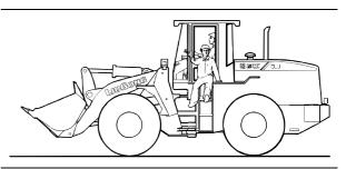
Before working the machine, you should operate the machine slowly to an open area, check for proper operation of all control levers and all protective devices.
