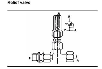
A---To pipe φ6 P---To pump unit R---Grease overflow
