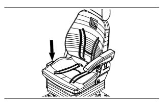
Three increment are available. When lifted to the max. height, the seat will get back to the min. height automatically.
