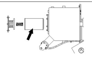
3. Replace with a new return oil filter element and O-ring. Install the return oil filter flange and oil drain plug. Hydraulic Oil Tank--Clean
