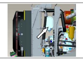
2. Unlock the four metal latches, and remove the cover of the air filter.
