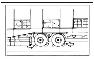
2. When the machine is loading on the trailer or truck, it is forbidden to turn.
