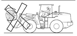
Do not use the bucket or boom for lifting. The machine can only be used within its capability. Any operation beyond its capability will bring damage to the machine. Refer to the Applications and Specifications section for the specific capacities.
