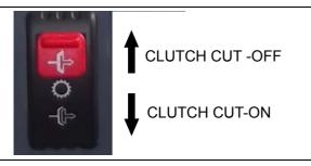
When the clutch cut off switch is turned to OFF, the power cut off function will be cancelled. That is, the transmission power output will not be cut off when the brake is engaged.
