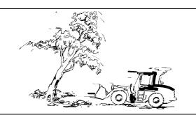
Consider filled or unstable ground. Be certain the condition of the work site is stable and capable of supporting the machine during operation. Do operate the machine close to an unstable drop off. Operation of the machine on shoulders, drop off's, or filled areas could cause the machine to become unstable, presenting a work hazard.
