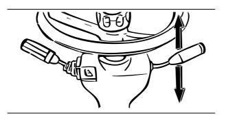
The high beam/ low beam can be achieved by the up and down movement as per the arrow direction.
