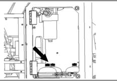
Accumulator 1 is used for the parking brake circuit and accumulator 2 and 3 are used for the service brake circuit.
