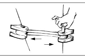
5. Loosen the bolt and adjust the bracket forward and backward to proper distance. Tighten bolt.
