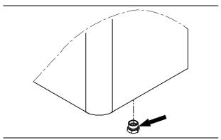
3. Remove the return oil filter end cap, take out the return oil filter element and O ring. Deal with them properly.
