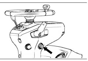
**OFF**——The oil passage of the engine is cut off at this position. The power of the machine is turned off. All of the other electrical appliances can not be turned on except the turn signal lights, rotating beacon and dome light.
