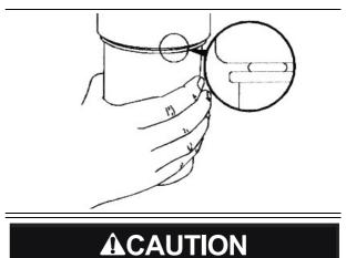
Keep the element clean during replacement to protect the pilot filter from being contaminated.
