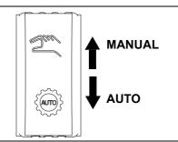
When AUTO is selected, the control box can shift the travel speed automatically by judging the engine speed and the current travel speed. When MANUAL is selected, the travel speed can only be shifted manually through the shift control lever.
