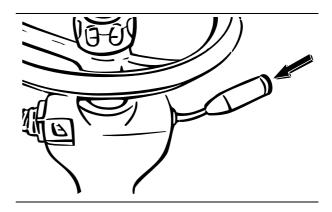
The horn will sound by pressing the horn button at the end of combination switch.
