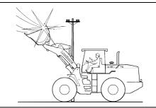
If the machine has contacted the high voltage wire:
