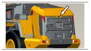
The camera will work after the monitor system is powered on. Ensure the operator has a good visibility during operation. The rear view mirror and mointoring system can help the driver with getting a good view of the rear side.
