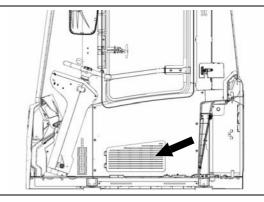
2. Clean the strainer with compressed air. If the strainer is too dirty or too oily, wash it with neutral detergent. Dry the strainer completely before reuse.
