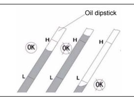
6. Reinsert the the oil dipstick and close the engine hood.
