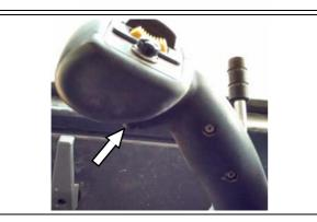
See above picture shows, the arrow direction is the operation direction of the KD key.
