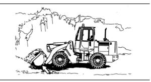
2. Apply down pressure to the bucket as the loader starts forward. Return the lift control to HOLD when sufficient penetration is obtained.
