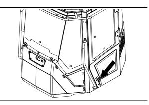
The machine cab only has one door on the left, and right side is window, the left door is installed with a door lock.
