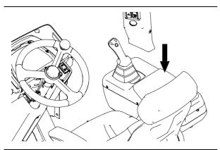
Loosen the mounting bolt of the hand pad support and move the hand pad up and down to appropriate position then tighten it.
