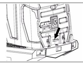
3. Open the engine hood in steps through releasing the rope in the middle of engine hood by hand until the engine hood fully open.
