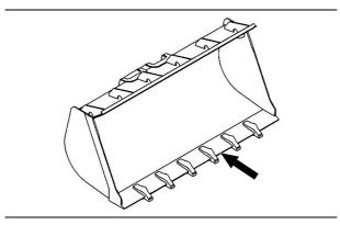
Check the cutting edges and the end bits for wear and for damage. Use the following procedure to service the cutting edges and the end bits:
