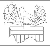
Check the coolant level only after the engine has been stopped and the coolant filler cap is cool enough to remove with your bare hand.
