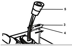
3. Nut 4. Stop plate 5. Pilot control lever
