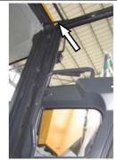
After the left door is opened to a particular opening, it can be opened completely and positioned automatically by an air spring, which is located on the top of the left door. Pull the inner handrail backward to close the left door.
