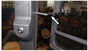
Extract the fixed pin to unlock the latch and then open the right window completely.
