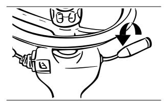
Front windshield wiper switch is located on the combination switch. There are four positions: OFF (O), intermittent (J), low velocity (I), high velocity (II). Rotate the switch to J position, the windshield wiper automatically works with low velocity at an interval of  $5\pm1s$ . Rotate the switch to I position, the windshield wiper works at low velocity, rotate it to II position, it works at high velocity.
