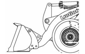
8. Tilt the quick coupler frame backward until the connecting pin aligns with pin hole of the work attachment.
