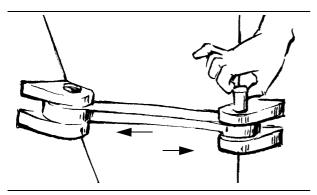
7. The lifting device should be fixed on the lift eyes with lift decals on the machine.
