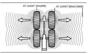
Dry nitrogen is recommended for inflation of tires. If the tires were originally inflated with air, nitrogen is still preferred for adjusting the pressure. Nitrogen mixes properly with air. Nitrogen inflated tires reduce the potential of a tire explosion because nitrogen does not aid combustion. Nitrogen helps to prevent oxidation of the rubber, deterioration of rubber, and corrosion of rim components.
