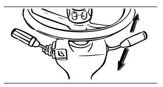
Push the combination switch forward when turning left, the left turn indicator will flash, and the front & rear left turn signal lights will also turn on simultaneously. Pull it backward when turning right, the right turn indicator will flash, and the front & rear right turn signal lights will also turn on simultaneously. When the hazard flasher switch is on, the turn signal lights will not work.
