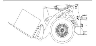
Travel with the material as low as possible while you still maintain ground clearance. Travel forward with the material uphill on upgrades and on downgrades. For better visibility, travel in reverse with bulky load.
