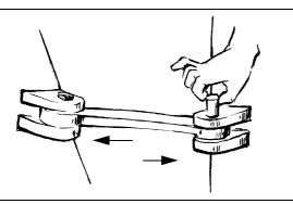
Loosen the bolts in following picture, adjust the bucket positioner switch in back and forth direction until it reaches proper position. Tighten the bolts.
