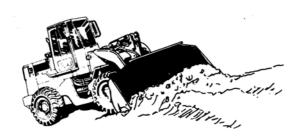
4. When the bucket is loaded, tilt it back against the stops. Carry the loaded bucket approximately 40 cm (15 inches) above the ground when moving to the dump area.
