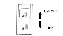
4. Loosen the nut of the auxiliary control lever lock and pull the stop plate outwards to unlock auxiliary control lever.
