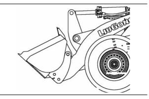
9. Pull the auxiliary control lever backward (to CLOSE position) to let the connecting pin of the quick coupler extends to connect with the work attachment.
