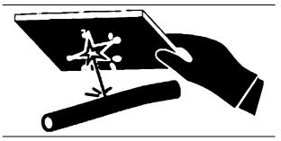
Even a pin-hole size leak can cause serious injury, If you are hit by spraying high-pressure oil, see a doctor for treatment at once.
