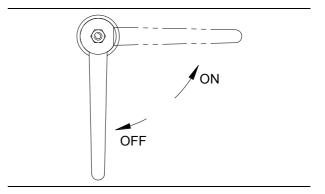
4. Install the steering frame lock.
