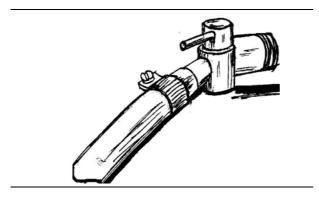
6. Open the filler cap of the water radiator recovery tank, slowly add coolant until the level reaches the filler cap of the recovery tank and keeps stable within 10 minutes.
