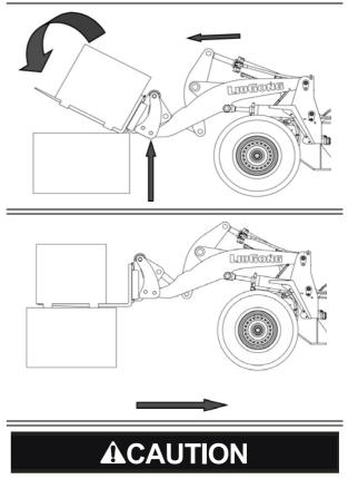
The level position of the forks top may change during this operation. Therefore, make sure that there is enough distance from the forks top to the material surface. 108 Operation Manual Engine Starting
