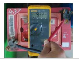
B) Observe the reading on the multimeter. The voltage value should be lower than 12.5V (lower than 25V if two batteries are measured in series), charge the battery in time. The states of voltage and electric charge are shown as below:
