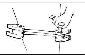
3. Remove the hexagonal plug at the bottom of the pilot filter and collect hydraulic oil with a suitable container.
