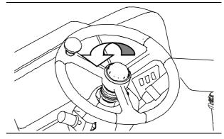
2. Rotate the adjusting handle clockwise for one quarter turn, the steering wheel will be locked, and it is unable to adjust the steering wheel upward or downward at this time.
