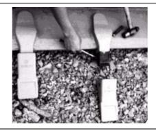
5. Install new tip on the tooth. Drive the pin into the snap ring, tooth, and tip from the side of the snap ring.
