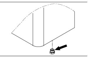
7. Meanwhile, open the breather filter cap (oil filler cap) of the hydraulic oil tank to quicken the oil discharging speed.
