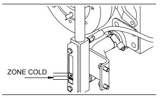
10. When the transmission oil reaches 80~90°C, check the oil level again. The level should be in the HOT ZONE of the sight glass. If the oil is insufficient, add oil. If the oil is excessive, drain some excessive oil.
