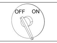
The battery disconnect switch and the engine start switch perform different functions. To disable the entire electrical system, turn the battery disconnect switch to the OFF position. The battery remains connected to the electrical system when you just turn off the engine start switch key.
