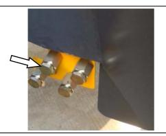
9. Remove the end cap of the return oil filter from the hydraulic oil tank, take out the return oil filter element and replace with a new one.
