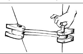
2. Press the parking brake button to disengage the parking brake.
