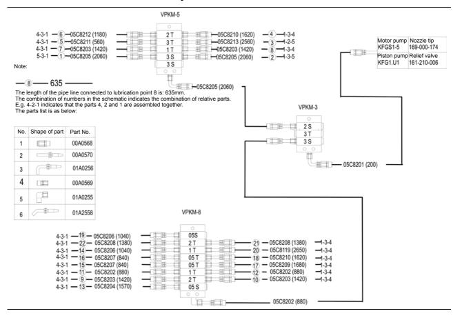
VPKM in the schematic is the step-forward controller, which is composed of several modules. The locations of VPKM-3, VPKM-5 and VPKM-8 are as shown below.
