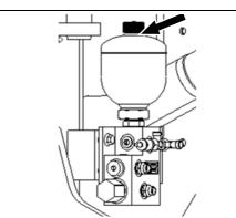
5. Tighten the valve A (rightward) on the accumulator charge tool, turn off the valve B then tighten the cap of valve C. Install the charge tool to the charge valve of the accumulator with slotted nut D.
