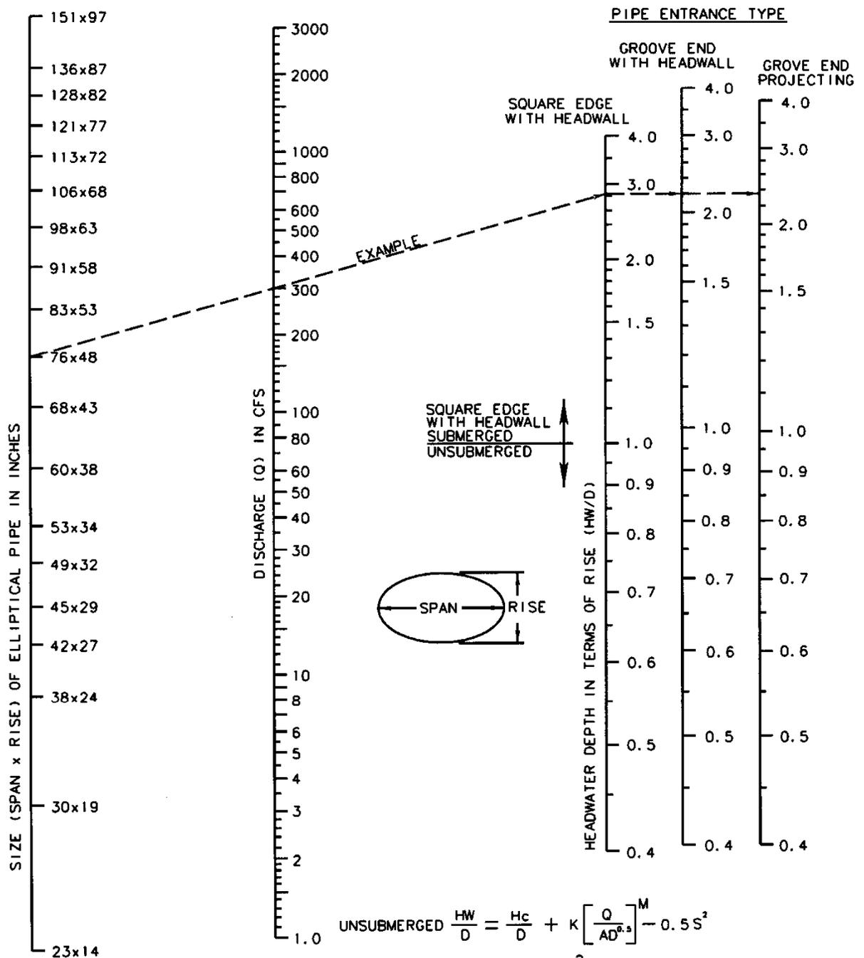
UNSUBMERGED  $\frac{HW}{D} = \frac{H_c}{D} + K \left[ \frac{Q}{AD^{0.5}} \right]^M - 0.5S^2$
