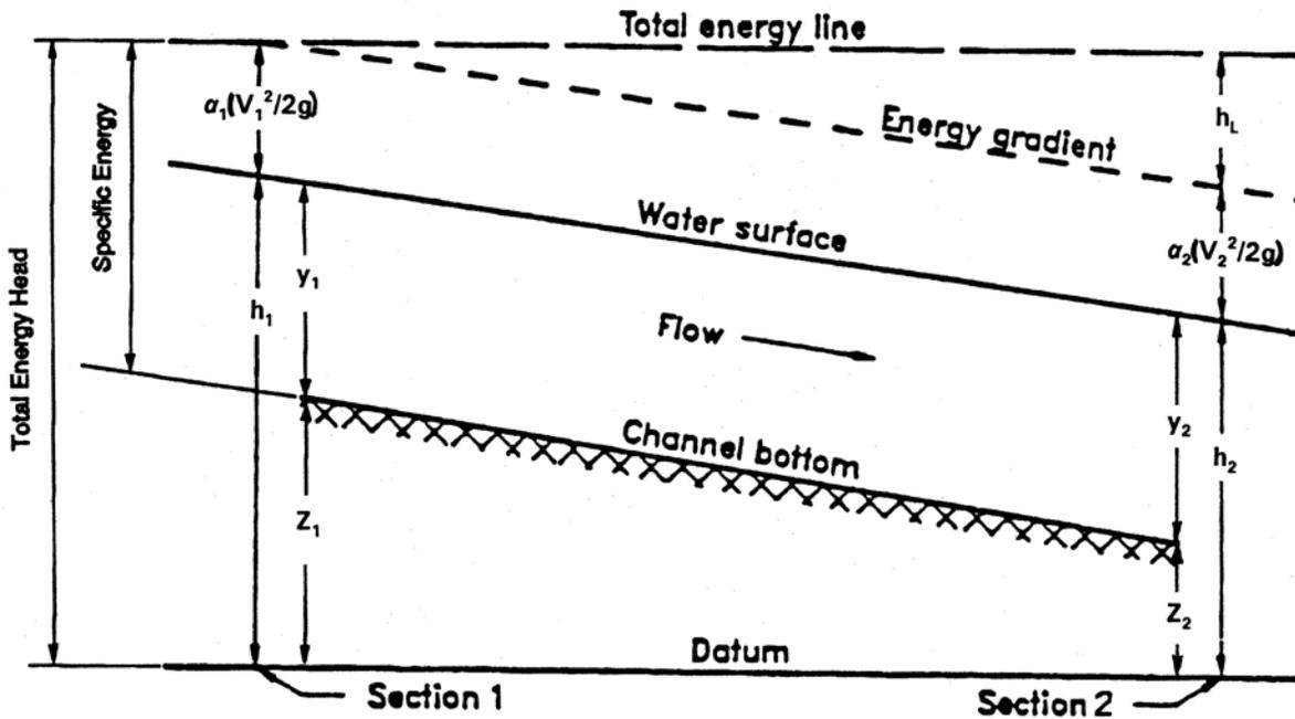
The total energy head is equal to the sum of the potential energy head (elevation head  $Z$  and pressure head  $Y$ ) and the kinetic energy head (velocity head  $V^2/2g$ ). The head loss is a measure of the *internal* energy dissipated in the whole mass of water due to friction with the channel boundary and minor losses due to changes in shape, cross sectional area and direction of flow between cross-sections.
