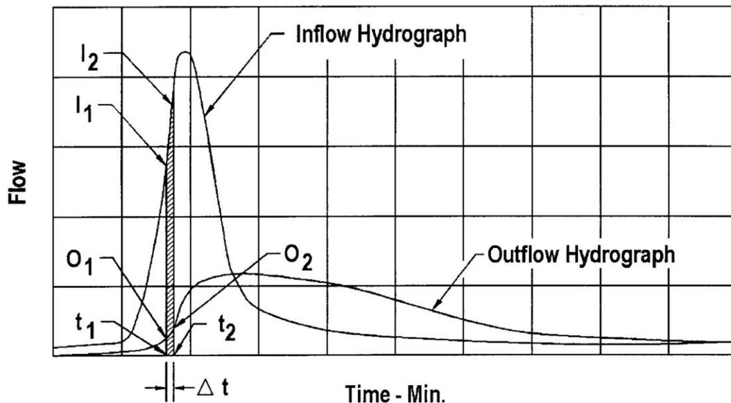
The equation can then be rearranged so that all the known values are on the left side of the equation and all the unknown values are located on the right side of the equation. Now the equation with two unknowns,  $S_2$  and  $O_2$ , can be solved with one equation.
