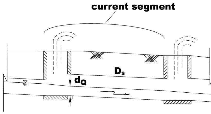
**$d_Q$  - water depth in inlet or access hole**
