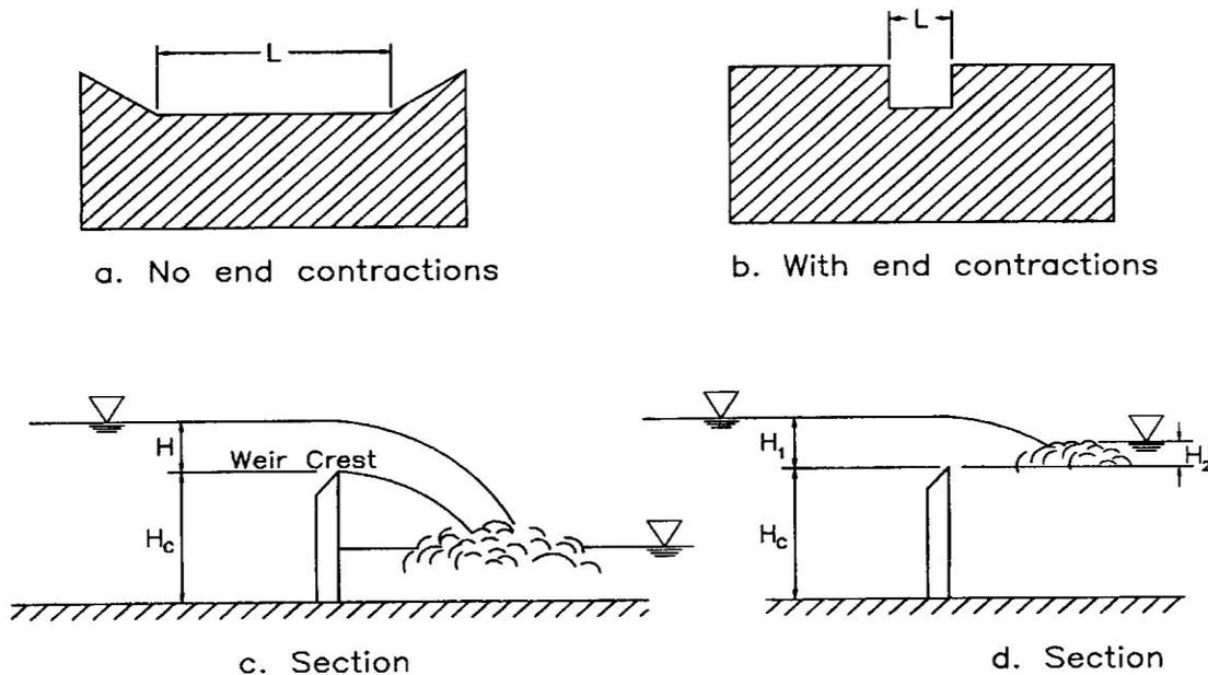
As indicated above, the value of the coefficient  $C_{SCW}$  is known to vary with the ratio  $H/H_c$  (see Figure 9-4c for definition of terms). For values of the ratio,  $H/H_c$  less than 0.3, a constant  $C_{SCW}$  of 3.33 is often used.
