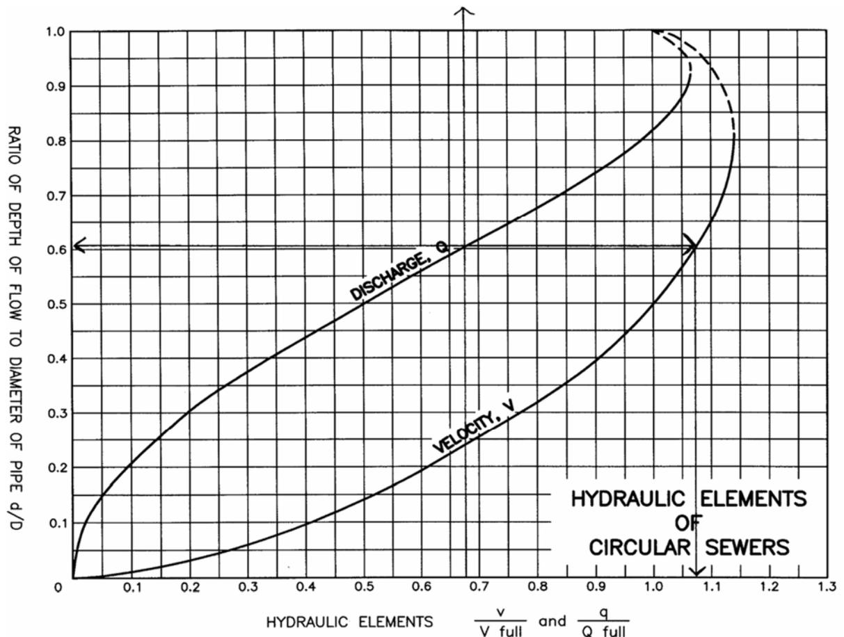
**Given:**  $D_{full} = 18$  in,  $Q = 7$  cfs (the design flow - i.e., what the actual flow will be under design conditions),  $V_{full} = 5.96$  fps (what the velocity would be at full flow),  $Q_{full} = 10.5$  cfs (what  $Q$  will be when the pipe is flowing full)
