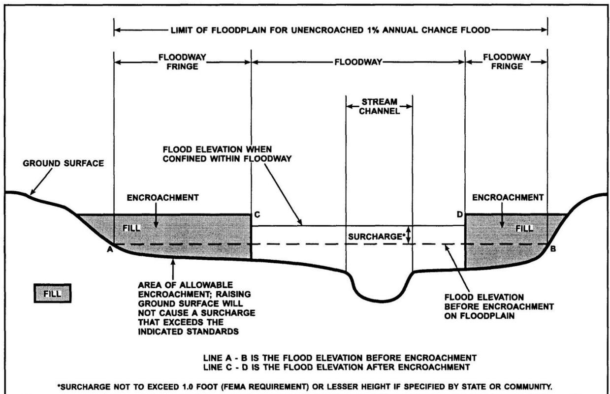
11. *Floodway Fringe*: The portion of the floodplain between the floodway boundary and the base flood boundary.
