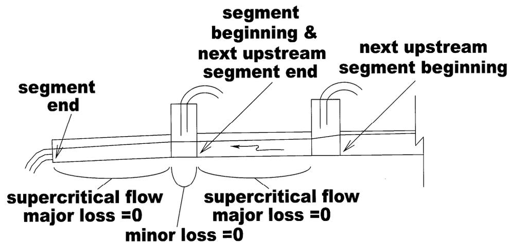
Therefore, if supercritical flow exists within the current segment pipe, the major loss is zero and column 31 shall be zero. If supercritical flow exists within the preceding segment pipe, the major loss for the preceding segment is zero and the minor loss for the structure in-between them shall also be zero.
