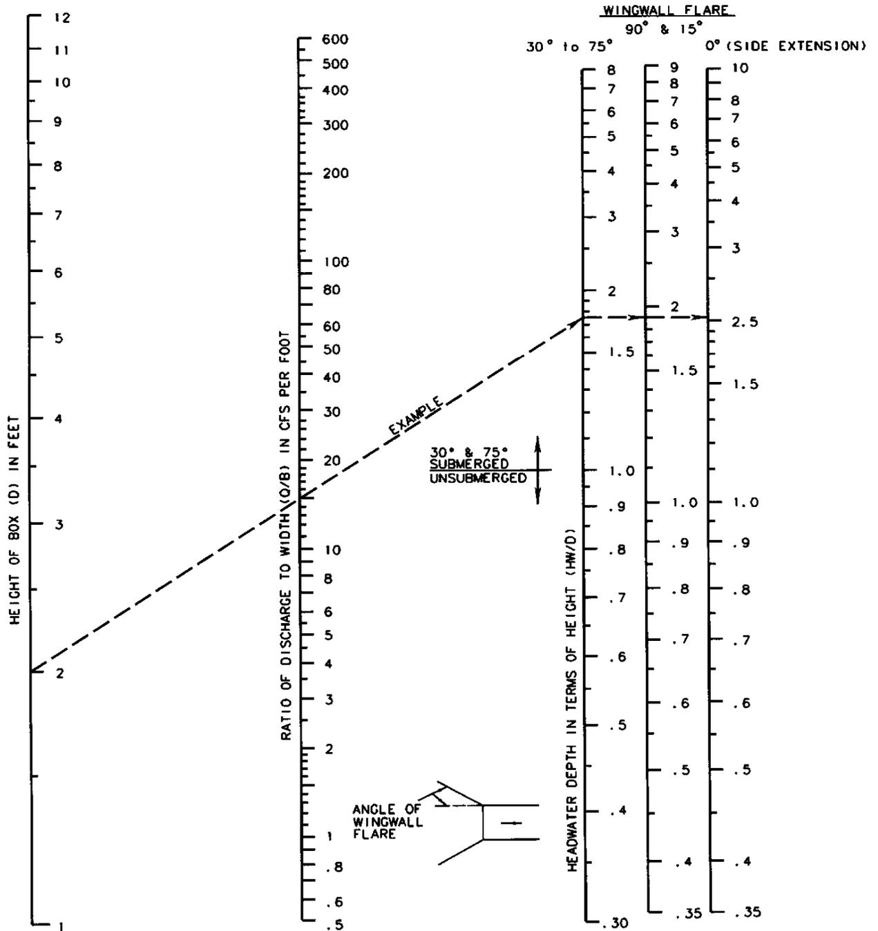
$$\text{UNSUBMERGED } \frac{HW}{D} = \frac{H_c}{D} + K \left[ \frac{Q}{AD^{0.5}} \right]^M - 0.5 S^2$$
