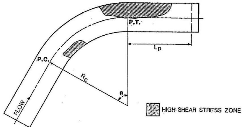
The increased shear stress caused by the bend persists a distance  $L_p$ , downstream of the bend. See Figure 7-6 for additional length of protection required.
