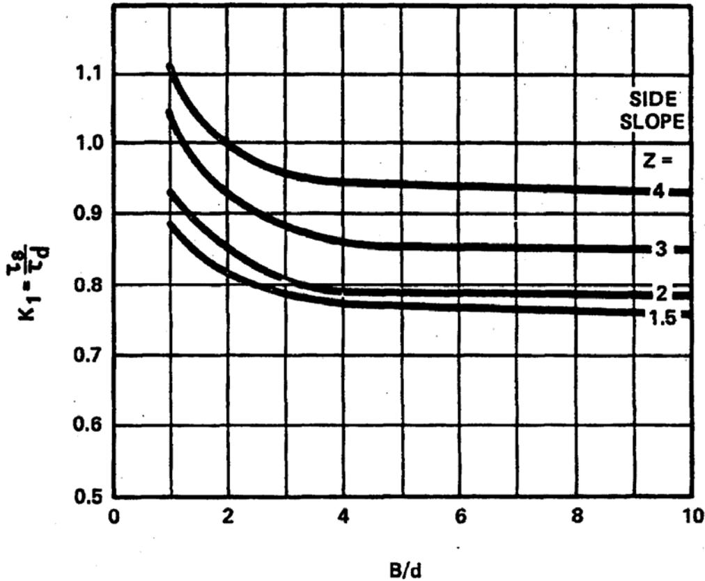
Source: *Design of Roadside Channels with Flexible Linings, HEC-15, FHWA, 1988*
