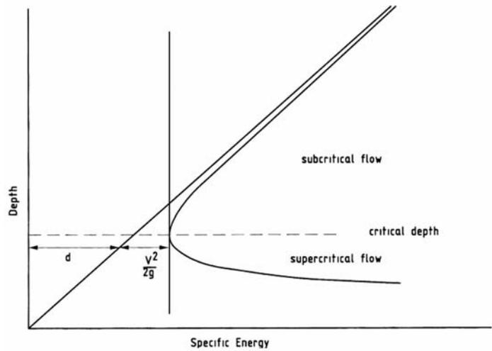
If we take small enough slices of our channel, the change in area with respect to the change in depth is equal to the water surface top width:
