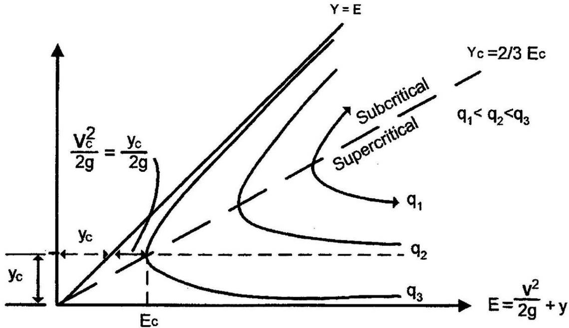
The specific energy diagram illustrates that normal depth can occur for subcritical, critical and supercritical flow conditions.
