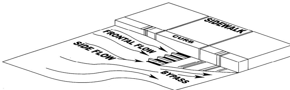
This ratio is equivalent to frontal flow interception efficiency or the ability of the inlet grate to accept the frontal flow approaching it. The average gutter velocity or total gutter flow divided by the gutter flow area is needed to calculate this ratio. Note that this ratio cannot exceed one. If it is equal to one, all of the flow is within the depressed gutter width and the grate is accepting the entire flow with no bypass.
