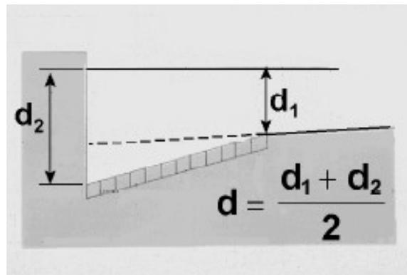
The capacity of a grate inlet operating as an orifice is:
