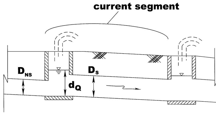
**$d_Q$  - water depth in inlet or access hole**
