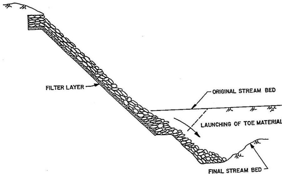
Source: *Design of Riprap Revetment, HEC-11, FHWA, 1989*
