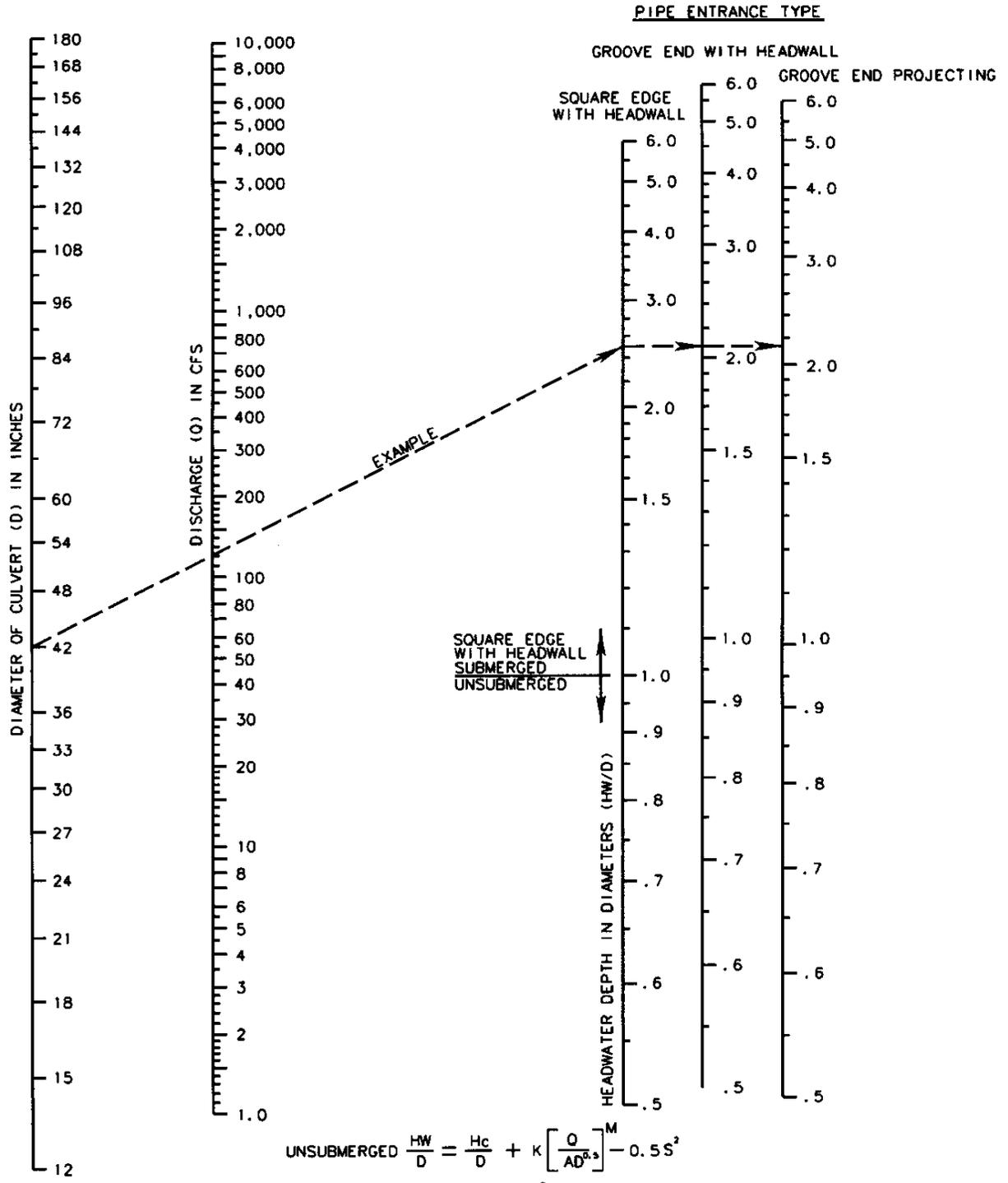
$$\text{UNSUBMERGED } \frac{HW}{D} = \frac{H_c}{D} + K \left[ \frac{Q}{AD^{2.5}} \right]^M - 0.5S^2$$
