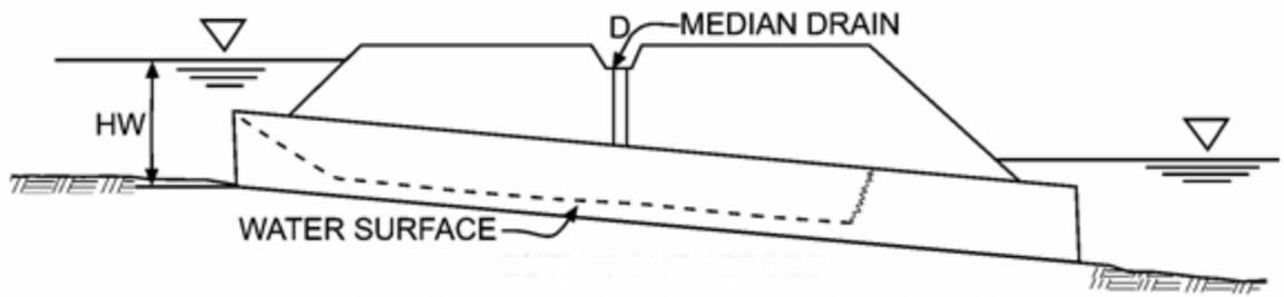
**INLET AND OUTLET SUBMERGED**
