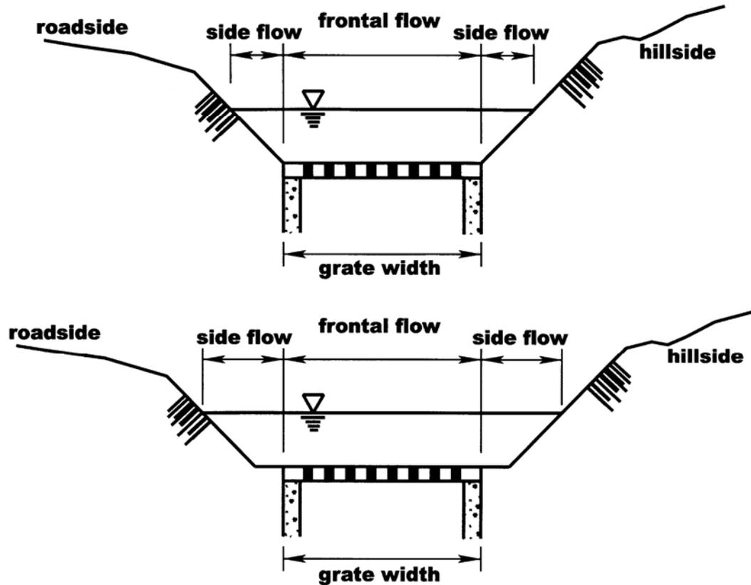
The interception efficiencies for frontal and side flow for Type G grates are obtained from Chapter 5, Chart 5-7 and Charts 5-8, respectively. The ratio of frontal flow to total gutter flow ( $E_o$ ) for a trapezoidal channel is shown in Chart 6-10 and obtained from the following equation:
