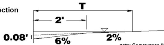
note: Conveyance (K) calc uses a mannings n = 0.013 for other values of n, multiply K by (0.013 / n). For spread over 8' use the formulas.
