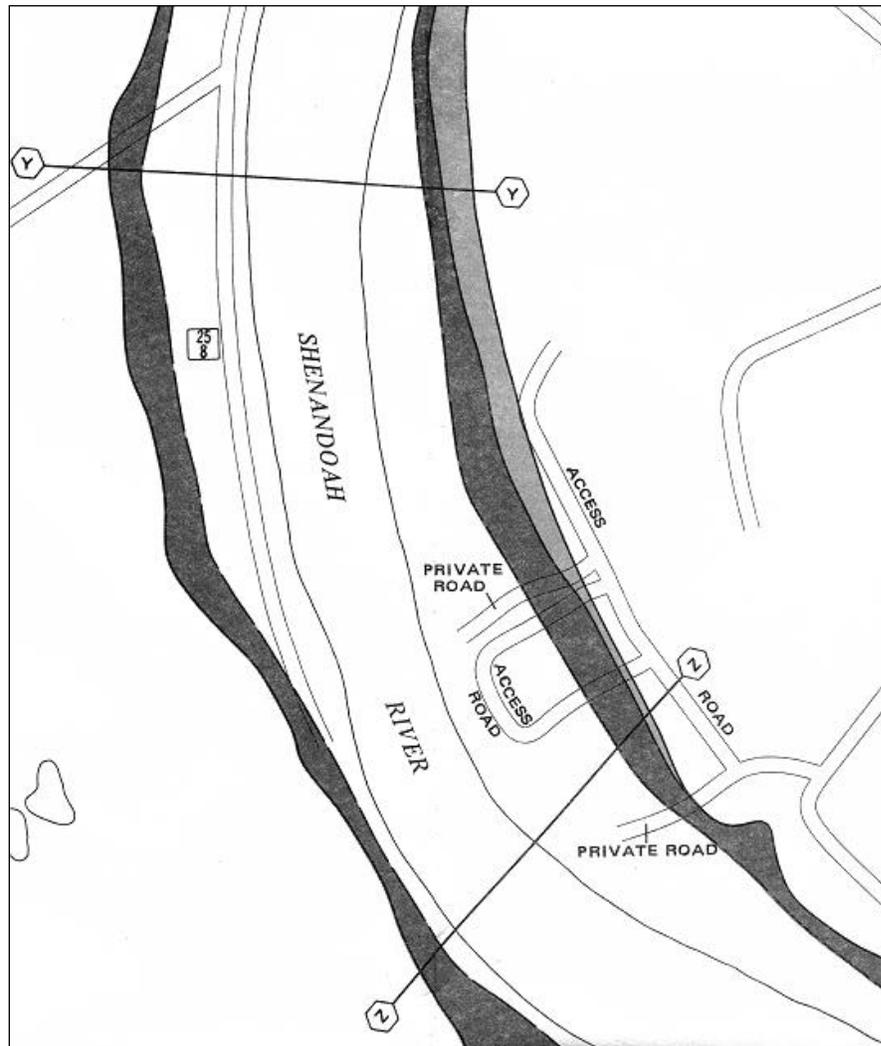
10. *Floodway*: A regulatory floodway adopted into a community's floodplain management ordinance, is the stream channel plus that portion of the overbanks that must be kept free from encroachments in order to discharge the base flood without increasing flood levels more than 1.0-foot (see Figure 10-4).
