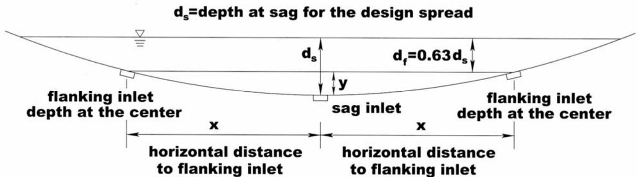
The following illustrates how the factor is determined if the flanking inlets are the same as the sag inlet:
