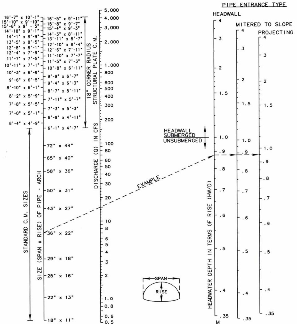
$$\text{UNSUBMERGED } \frac{HW}{D} = \frac{H_c}{D} + K \left[ \frac{Q}{AD^{0.5}} \right]^M - 0.5S^2$$
