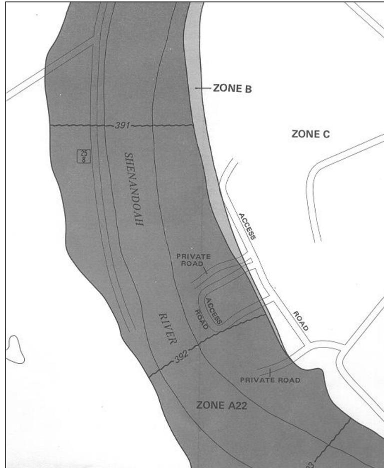
Base Flood Elevations (BFEs) are shown as wavy lines across the base floodplain.
