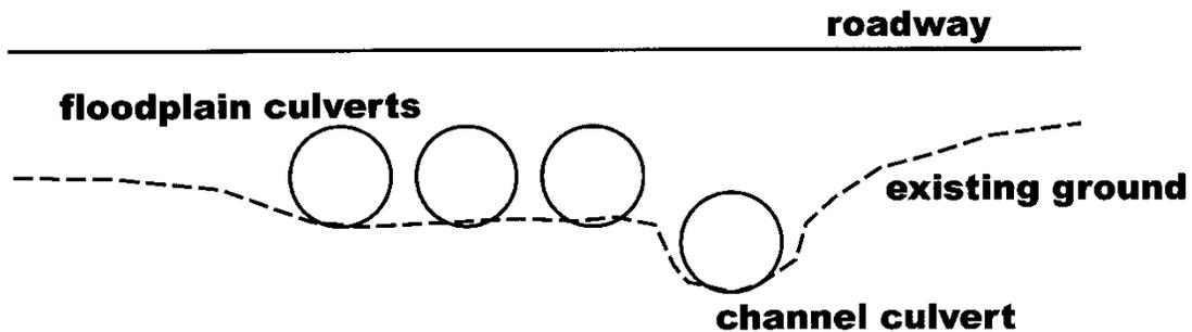
The designer is cautioned that multiple cell culverts are not appropriate for all streams; therefore a stream stability assessment must be conducted to determine if they are appropriate. Multiple cell culverts should be considered only on stable streams that have active floodplains. A bridge is more appropriate for unstable streams or streams with no floodplain.
