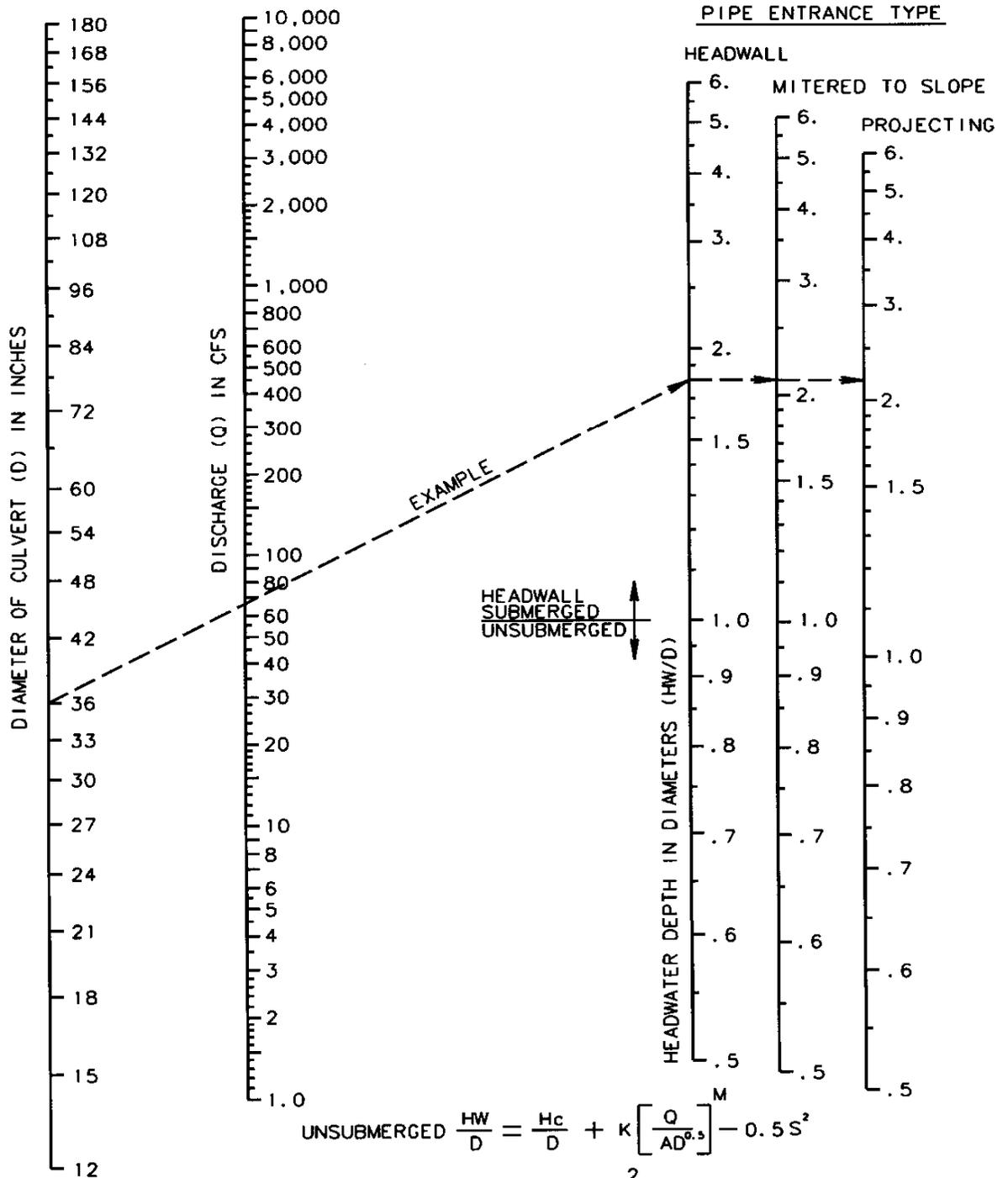
UNSUBMERGED  $\frac{HW}{D} = \frac{H_c}{D} + K \left[ \frac{Q}{AD^{0.5}} \right]^M - 0.5S^2$
