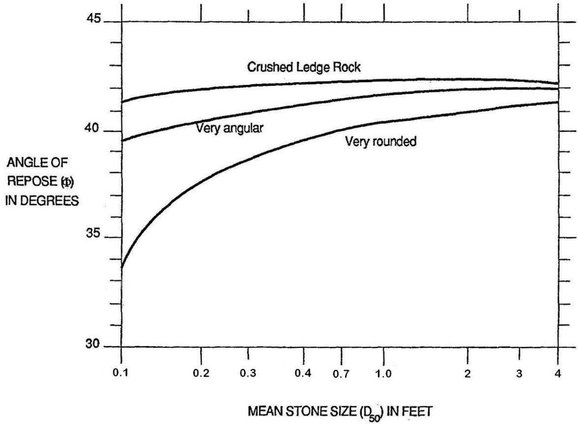
Source: *Design of Riprap Revetment, HEC-11, FHWA, 1989*
