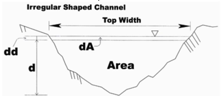
Depth of flow determines the flow area (A) and the flow top width (T). To solve for critical depth, find the flow (Q) and its corresponding depth (d) that create the equality in this equation.
