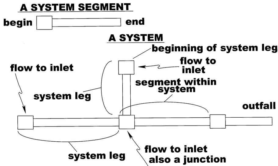
**STEP 1, PIPE ID:** Start at the beginning of a system leg on line 1. Fill in column 1 (FROM POINT) with the inlet label from the plan sheet. Fill in column 2 (TO POINT) with the proceeding inlet label from the plan sheet. All legs attached to the next segment shall be designed before continuing on to a segment within the system (legs 2-3 and 1-3 in the diagram on the next page).
