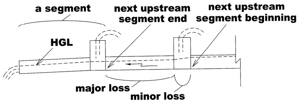
Hydraulic grade line computations begin at the outfall of the system and are calculated upstream taking each junction into consideration.
