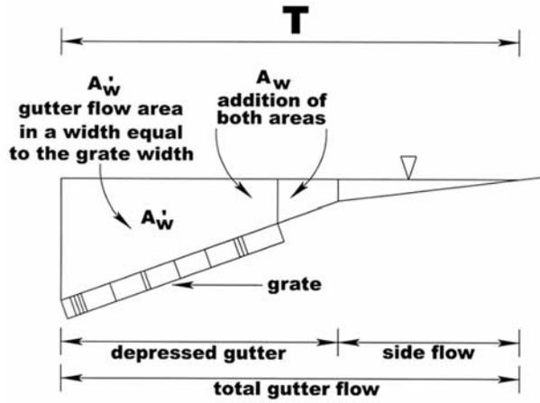
The ratio of side flow to total gutter flow ( $Q_s/Q$ ) is:
