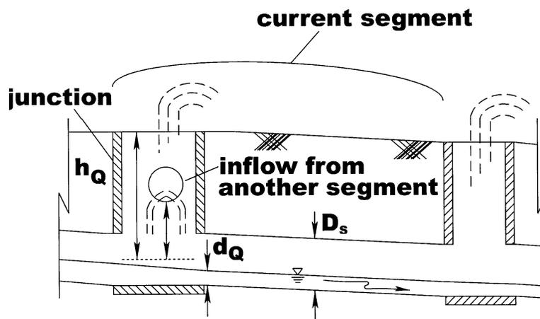
**$d_Q$  - water depth in inlet or access hole**
