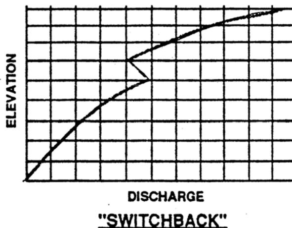
This phenomenon can occur in any type of conveyance computation, including the step-backwater method. Computer logic can be seriously confused if a switchback were to occur in any cross-section being used in a step-backwater program. For this reason, the cross-section should always be subdivided with respect to both vegetation and geometric changes. Note that the actual *n*-value, itself, may be the same in adjacent subsections.
