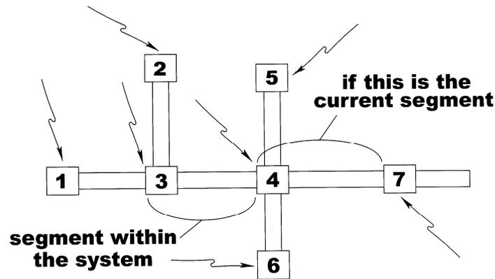
Compare the column 21 values for segment 3-4, segment 5-4, and segment 6-4 to the time of concentration into inlet 4 and record the largest value in column 7 for the current segment.
