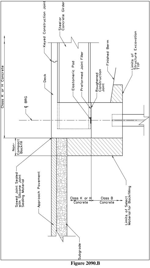
INTEGRAL ABUTMENT FOR DECK-GIRDER SYSIEM (WITHOUT APPROACH SLAB)
