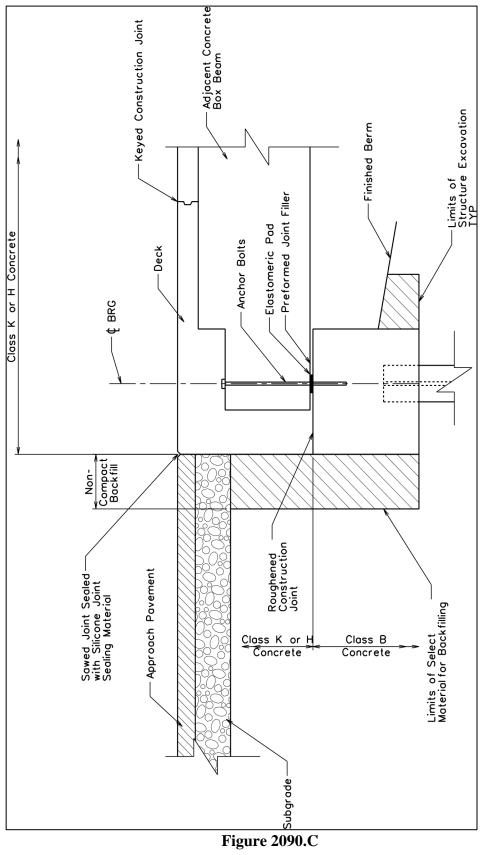
INTEGRAL ABUTMEN - 03 ADJACEN CONCRETE BOX BEAMS (WITHOUT APPROACH SLAB)
