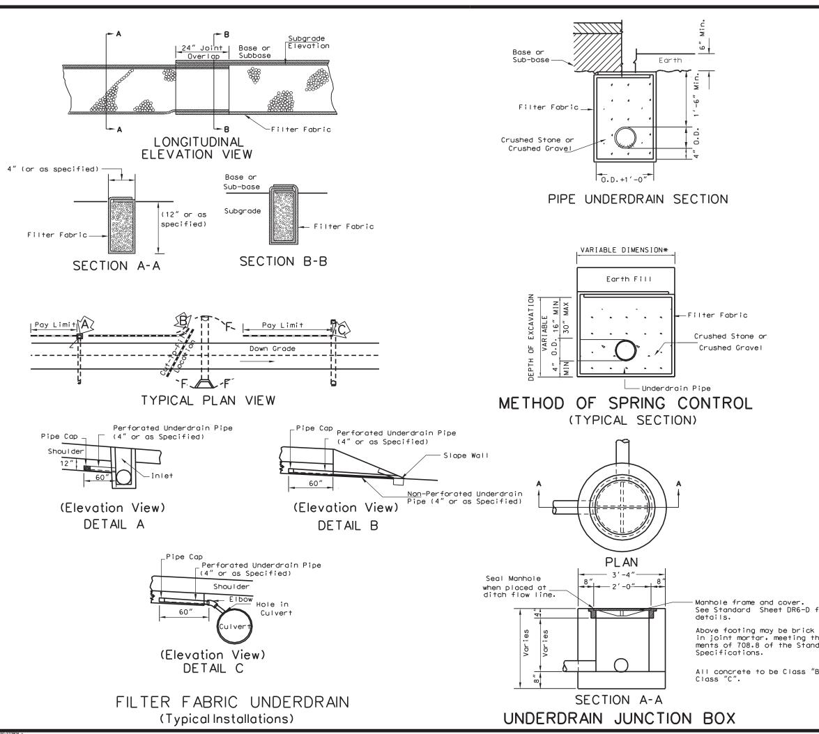
Filter fabric and aggregate for filter fabric underdrain shallconform to the requirements of Section 606.2 of the Specifications. All costs associated with the 5' perforated Underdrain pipe required in the Filter Fabric Underdrain installation to be included in the contract price bid for Filter Fabric Underdrain.
