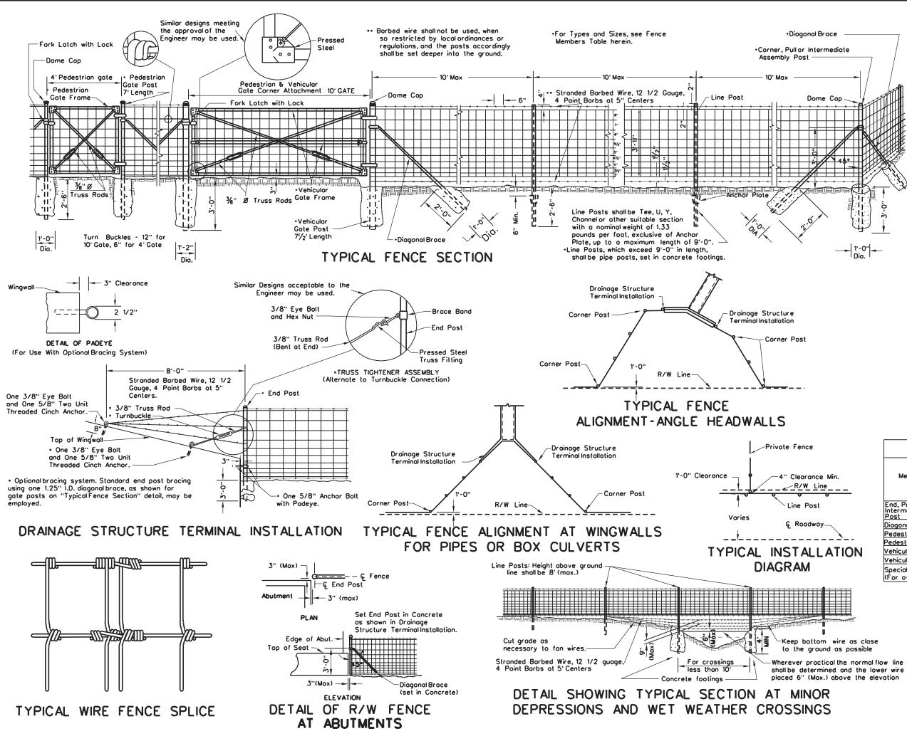
Except for "normal length" line posts, all other posts and their diagonal braces shall be either galvanized steel pipe members or triple -coated steel pipe members as shown in the "Fence Members Table" herein. When galvanized pipe posts are used, galvanized pipe diagonal braces shall be used. When triple-coated pipe posts ore used, triple-cooted pipe diagonal braces shall be employed
