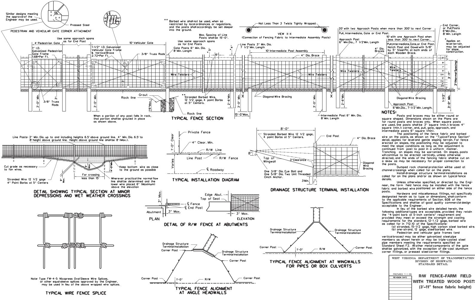
fabric and barbed wire positioned on either side of the fence
