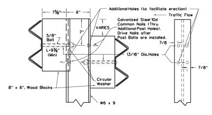
STEEL GUARDRAIL POST (WOOD BLOCK) (BEAMS AT DIFFERENT ELEVATIONS)
