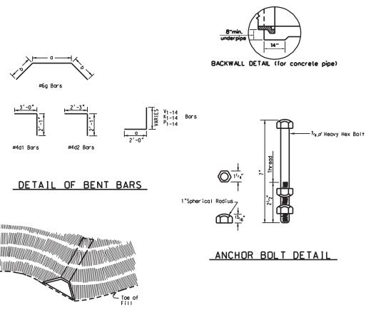
SKEWED PIPE CONSTRUCTION DETAIL
