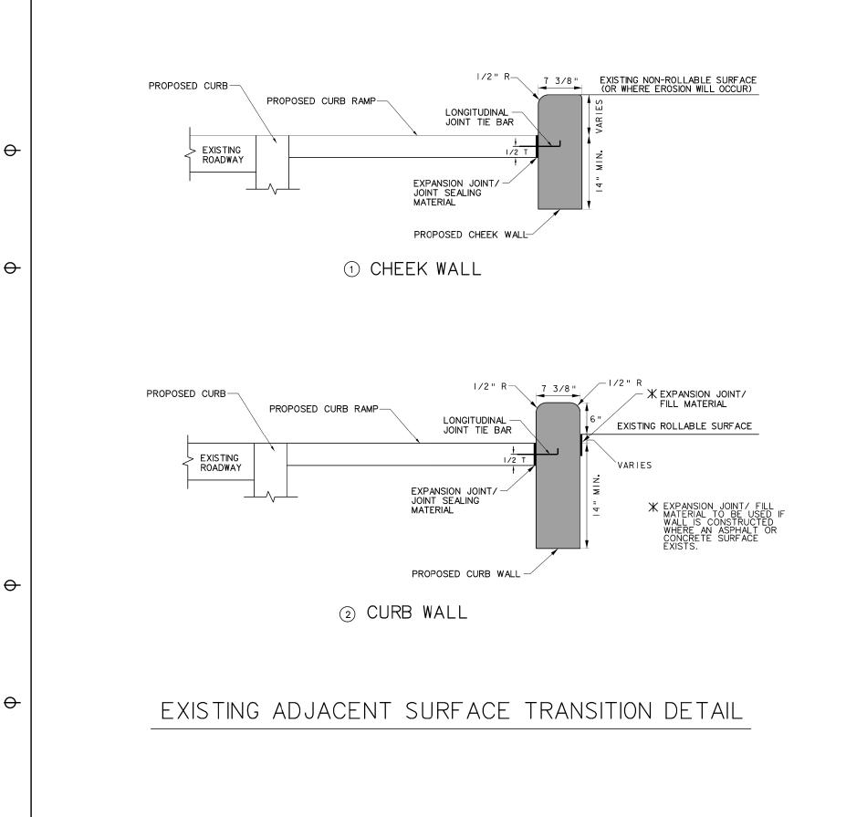
PAY LIMITS FOR PROPOSED ADJACENT SURFACE TRANSITION DETAIL (INCIDENTAL TO 609005-\* CURB RAMP)
