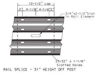
Eight (8) Splice Bolts are to be used at all Rail Splices
