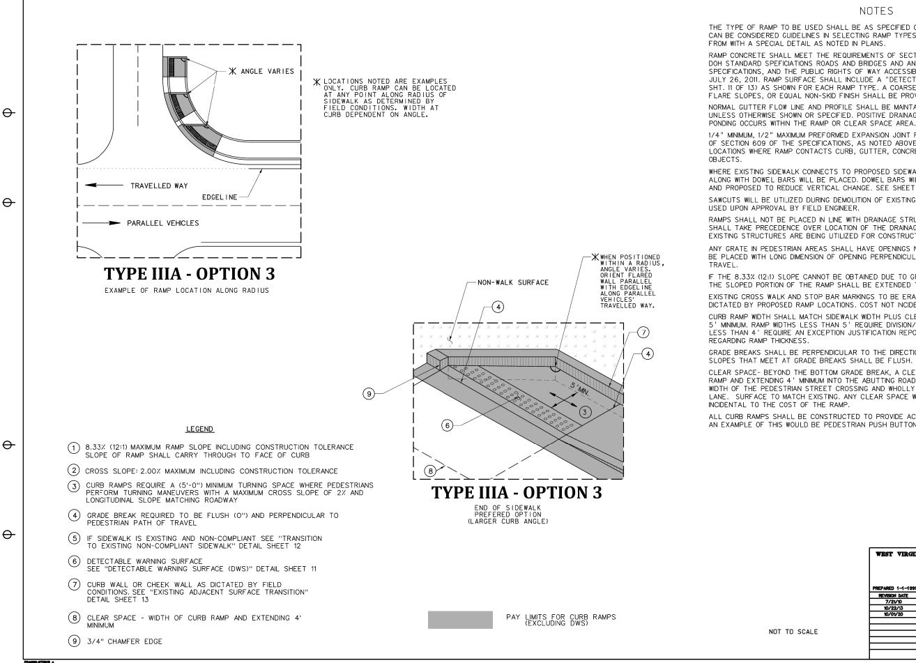
THE TYPE OF RAMP TO BE USED SHALL BE AS SPECIFIED ON THE PLANS. THESE STANDARDS CAN BE CONSIDERED GUIDELINES IN SELECTING RAMP TYPES, HOWEVER THEY CAN BE DEVIATED
