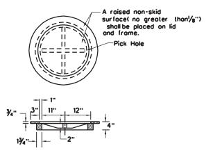
DETAIL OF FRAME AND COVER CASTING (RING TYPE)
