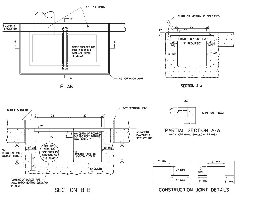
FOR DETAILS OF GRATE SUPPORT BAR, SHALLOW FRAME, AND GRATES (TWO REQUIRED), SEE INLET CASTINGS STANDARD SHEET DR6-X. USE OF THE SHALLOW FRAME WILL BE LIMITED TO ROADWAYS CONSTRUCTED OF CONCRETE PAVEMENT. IF ADJACENT ROADWAY IS BUILT OF HOT MIX ASPHALT PAVEMENT, THE FRAME AS REQUIRED FOR A TYPE F INLET (STANDARD SHEET DR6F) WILL BE REQUIRED.
