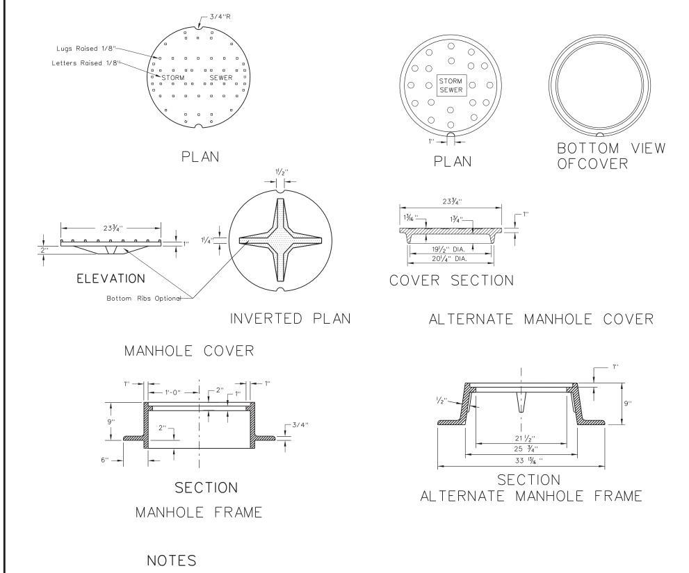
Lettering on covers shall denote STORM SEWER or SANITARY SEWER as applicable.
