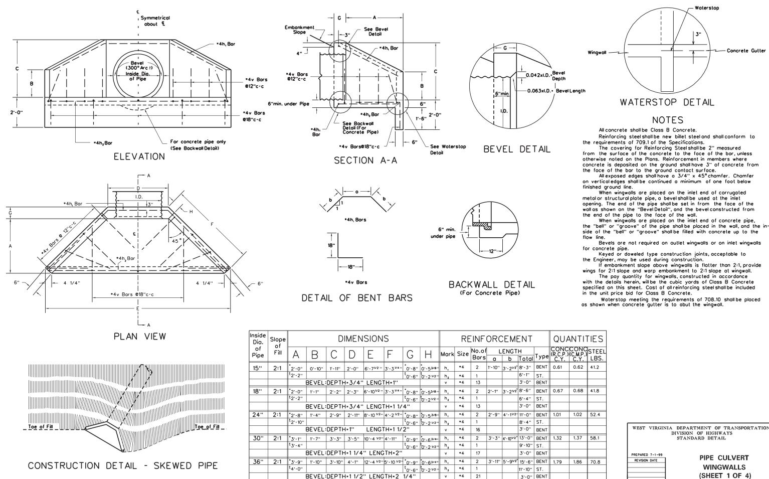
\* DIMENSIONS FOR INLET WINGWALLS ON CORRUGATED METAL PIPE (TO ACCOMMODATE THE BEVEL). t DIMENSIONS FOR INLET WINGWALLS ON CONCRETE PIPE AND ALL OUTLET WINGWALLS.
