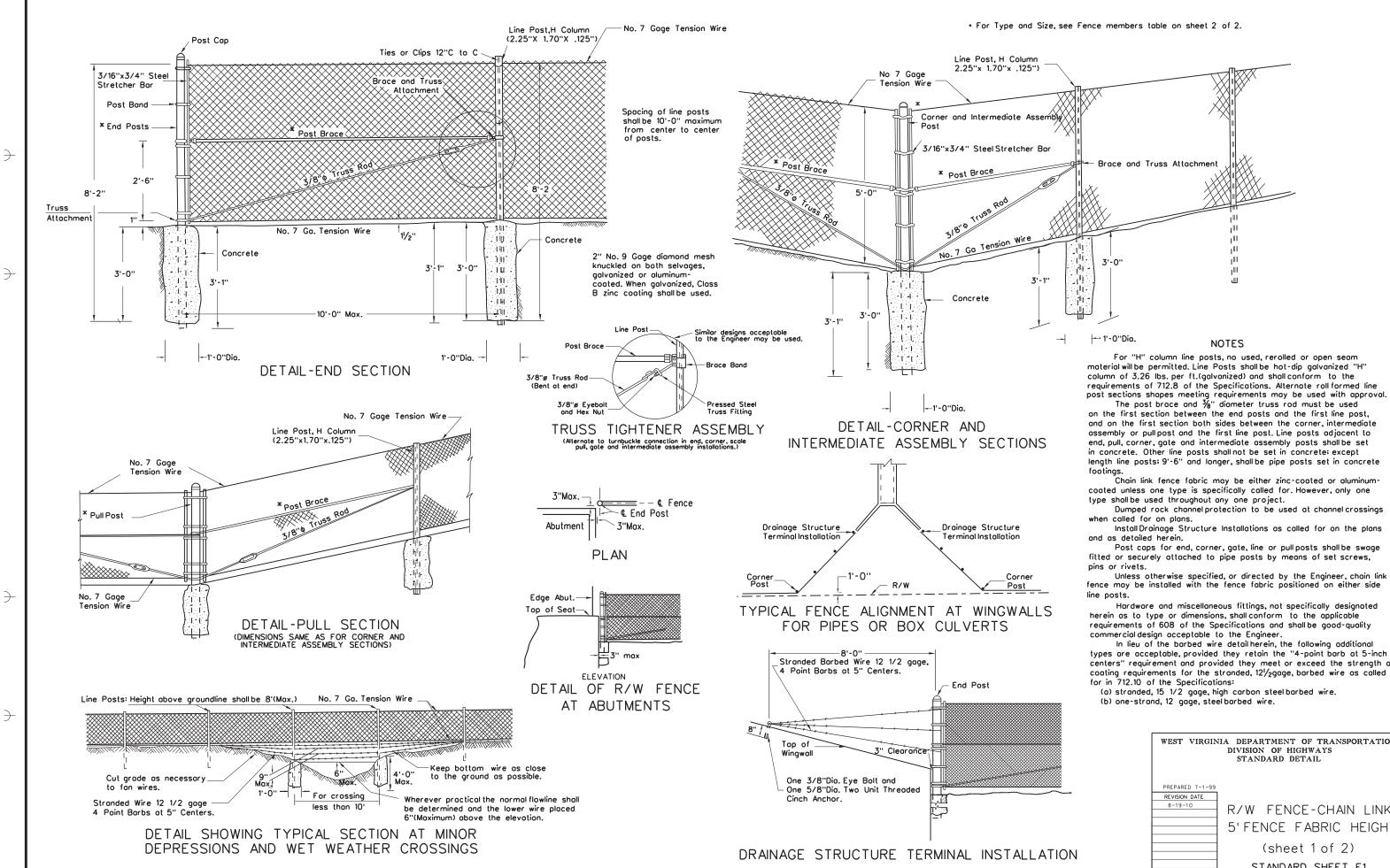
For "H" column line posts, no used, recolled or open seam material will be permitted. Line Posts shall be hot-dip galvanized "H" column of 3.26 lbs. per ft.(galvanized) and shall conform to the
