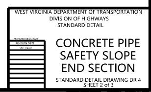
CONCRETE TO BE 3200 PSI MINIMUM COMPRESSIVE STRENGTH AT 28 DAYS. ALL REINFORCING STEEL TO CONFORM TO THE REQUIREMENTS OF 709.1 AND 709.4 OF THE SPECIFICATIONS. THE COST OF CONCRETE, STEEL REINFORCING, ALL OTHER REQUIRED ITEMS, SUCH AS, GASKET, GROUT, BEDDING, BACKFILL MATERIAL, PLACEMENT, ETC. IS INCLUDED IN THE COST OF THE CONCRETE PIPE SAFETY SLOPE END SECTION.
