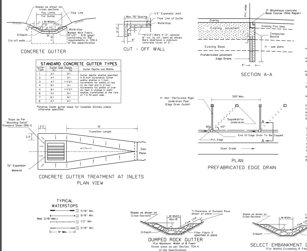
Waterstop shall be 5" wide min; web min. thickness  $\%_6$  ; end section and / or ribs less than 1.67 web thickenss.
