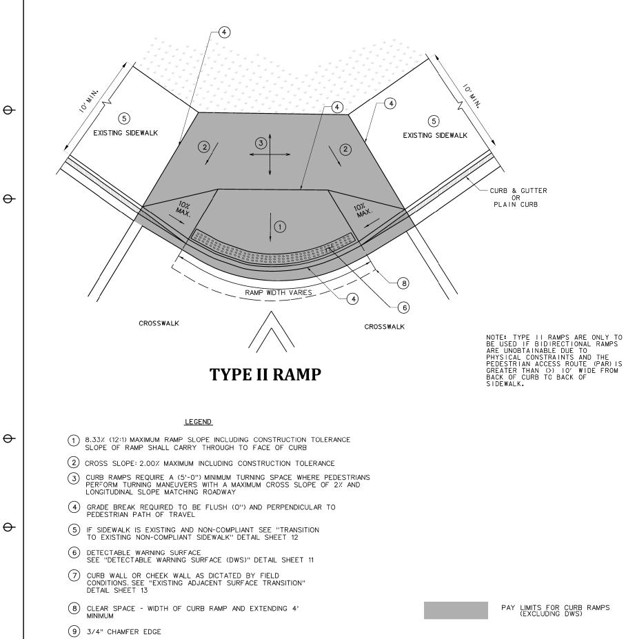
THE TYPE OF RAMP TO BE USED SHALL BE AS SPECIFIED ON THE PLANS. THESE STANDARDS CAN BE CONSIDERED GUIDELINES IN SELECTING RAMP TYPES. HOWEVER THEY CAN BE DEVIATED FROM WITH A SPECIAL DETAIL AS NOTED IN PLANS.
