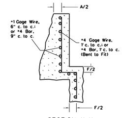
SECTION X-X (Showing Reinforcing Details)
