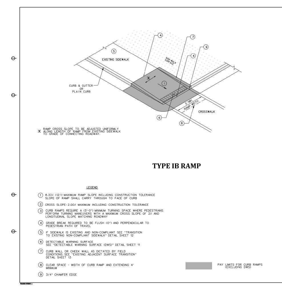
THE TYPE OF RAMP TO BE USED SHALL BE AS SPECIFIED ON THE PLANS. THESE STANDARDS CAN BE CONSIDERED GUIDELINES IN SELECTING RAMP TYPES, HOWEVER THEY CAN BE DEVIATED FROM WITH A SPECIAL DETAIL AS NOTED IN PLANS.
