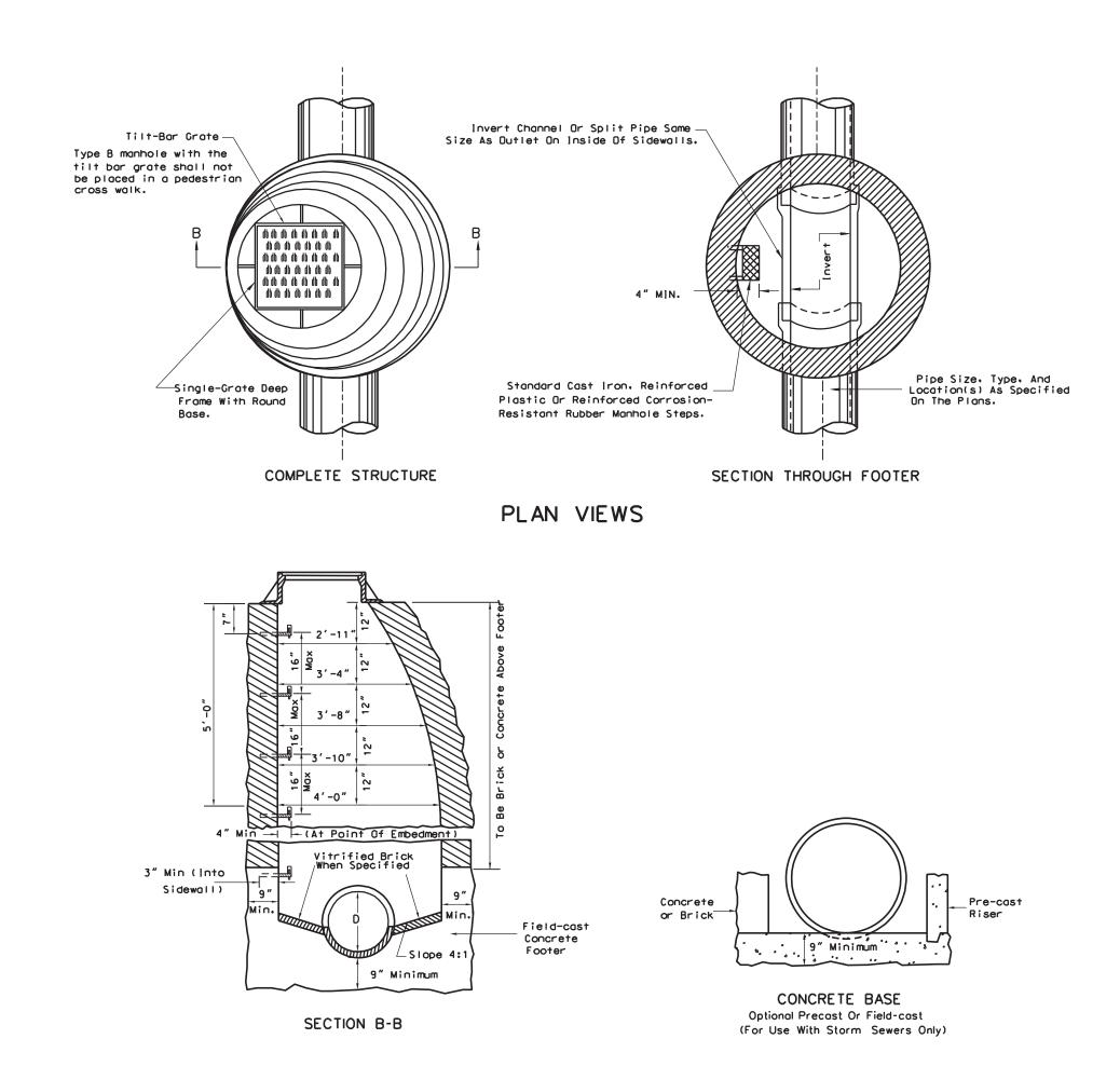
"Keyed" Or "Doweled" Type Construction Joints, Acceptable To The Engineer, May Be Used In The Construction Of Concrete Manholes.
