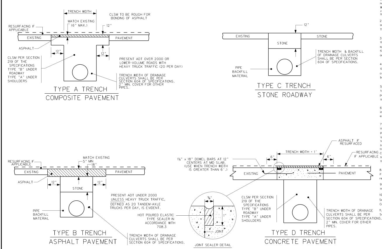
1. The type of backfill and repaving of trenches under existing pavement shall be as specified in the plans. If no type is specified, the applicable detail shall be used. When a Type F Trench is specified under an existing roadway, repaving of the pavement section shall be per the applicable detail on this sheet.
