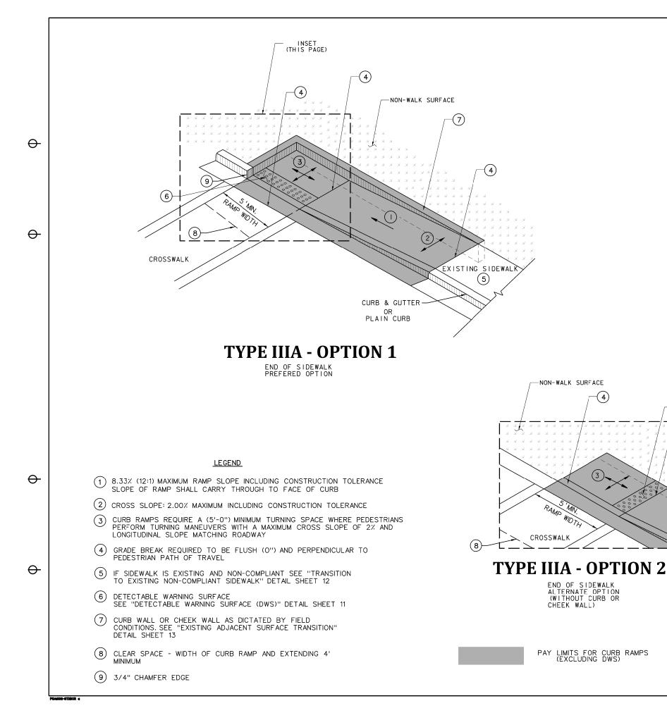
THE TYPE OF RAMP TO BE USED SHALL BE AS SPECIFIED ON THE PLANS. THESE STANDARDS CAN BE CONSIDERED GUIDELINES IN SELECTING RAMP TYPES, HOWEVER THEY CAN BE DEVIATED FROM WITH A SPECIAL DETAIL AS NOTED IN PLANS.
