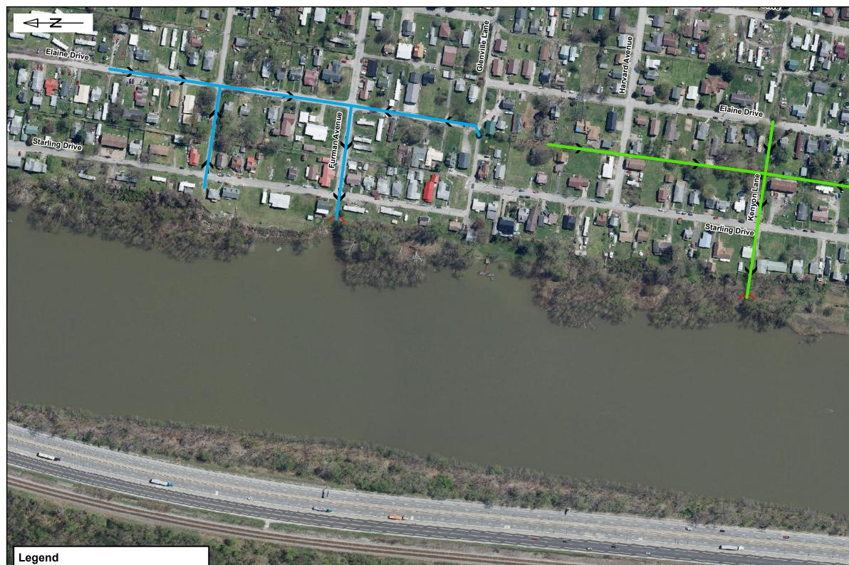
Construction Phases (Phase 1 & 2 ONLY) Phase 1 Phase 2 **Flow Direction** ← North → South 个 East  $\mathbf{J}$ West Outfall Type New Outfall
