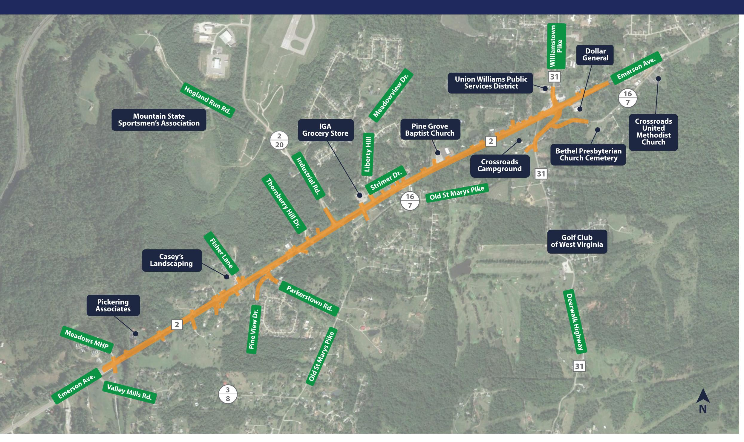
The new roadway will be similar to the roadway that has already been constructed. It will provide two northbound lanes, two southbound lanes, a continuous center turn lane and paved shoulders. Roadway widening will continue along the right side of the roadway until it approaches WV 31. The roadway will transition back to the existing two lane configuration north of WV 31.
