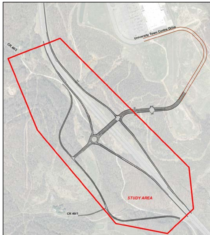
Diamond Interchange with Roundabout at southbound ramps
