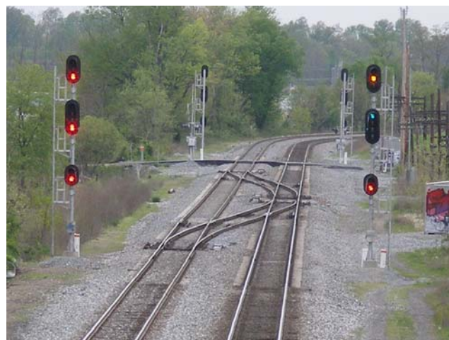
Example of Rail Interlocking
