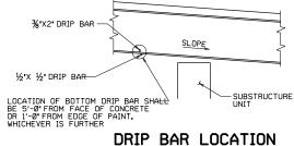
DRIP BARS SHALL BE LOCATED ON THE UPWARD SLOPE OF ALL GIRDERS ADJACENT TO SUBSTRUCTURE UNITS.
