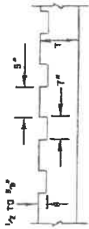
ALTERNATE SECTION 8-8 (SAVED RUMBLE STRIP)
