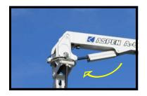
Turntable no. 2 comes equipped with an automatic leveling system, providing smooth platform movement. In addition, the operator can make manual adjustments of  $\pm$ 0 degrees to compensate for the slope of the bridge. With the elimination of the leveling arms, the Aspen A-62 has more vertical clearance to get over high fences.
