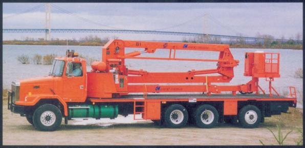
The Model UB50 in the traveling position.
