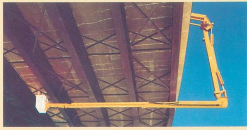
EXTENDED REACH - Up to 60' (18.3 m) of underbridge working reach available without requiring that the truck chassis be repositioned.
