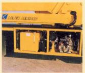
TWO POWER SOURCES are provided. The primary source of power is a power-take-off from the truck transmission. A liquid-cooled diesel engine capable of powering the Bridge Inspection Unit is provided as backup.
