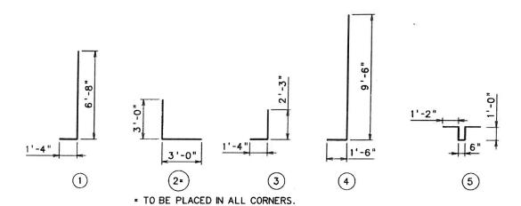
BENT REBAR DETAIL
