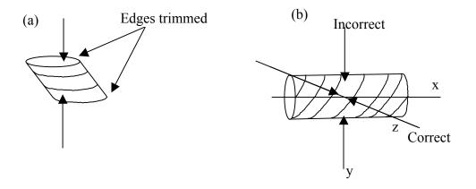
Figure 6: Loading directions for test on anisotropic rock.
