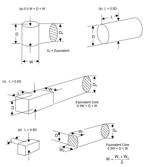
Figure 6.1: Load Configurations and Specimen Shape Requirement for (a) the Diametral Test, (b) the Axial Test, (c) the Block Test, and (d) the Irregular Lump Test.
